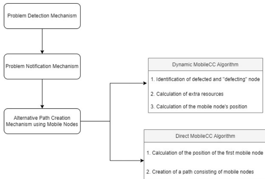
**Figure 1.** Block Diagram of the Framework.
