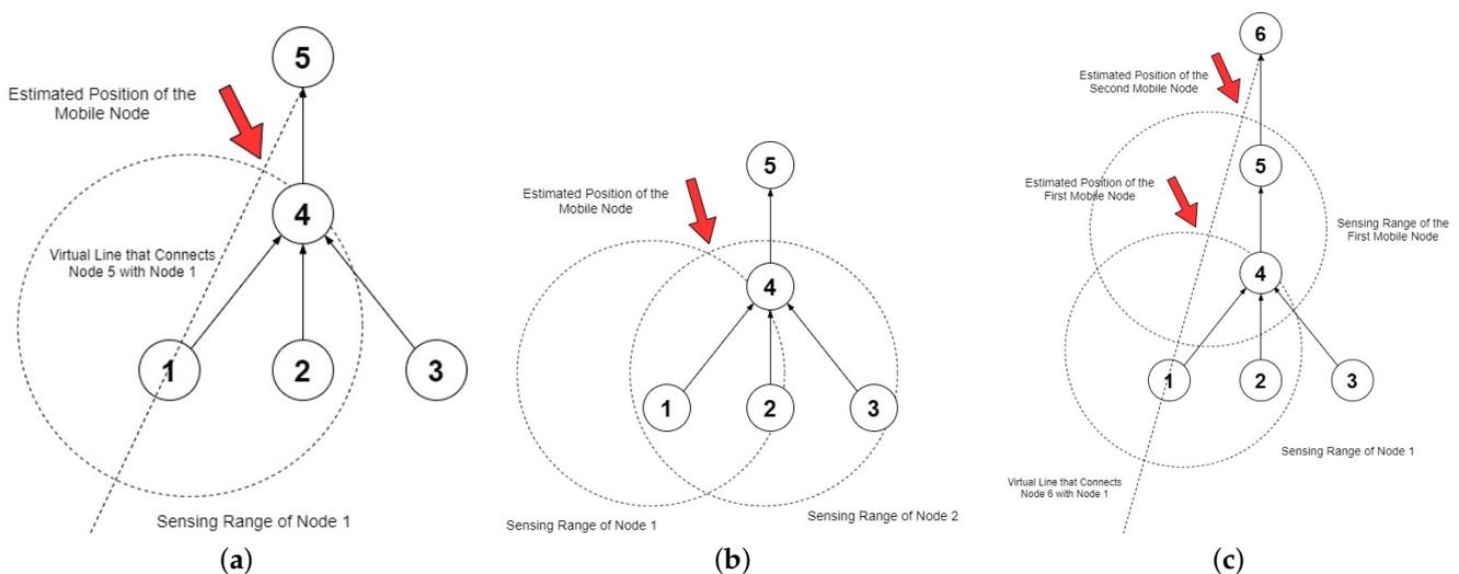
**Figure 2.** Node Placement Positions [8]. (a) Single Node, (b) Multiple Node, (c) Direct Path.
