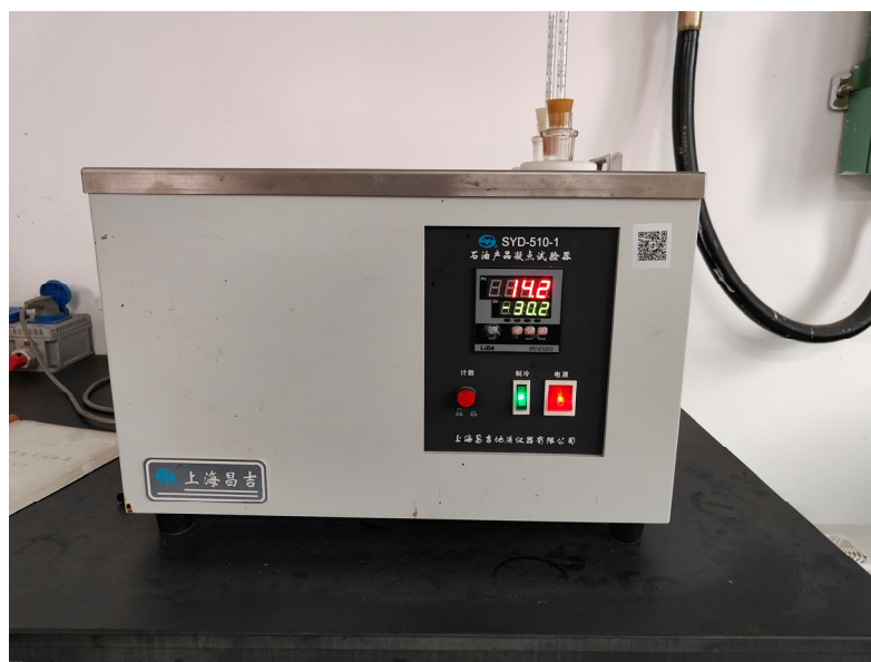
Figure 1. Experimental setup for measuring the pour point of oil products. The Chinese characters marked on the equipment represent the official brand and model name of the experimental instrument.
