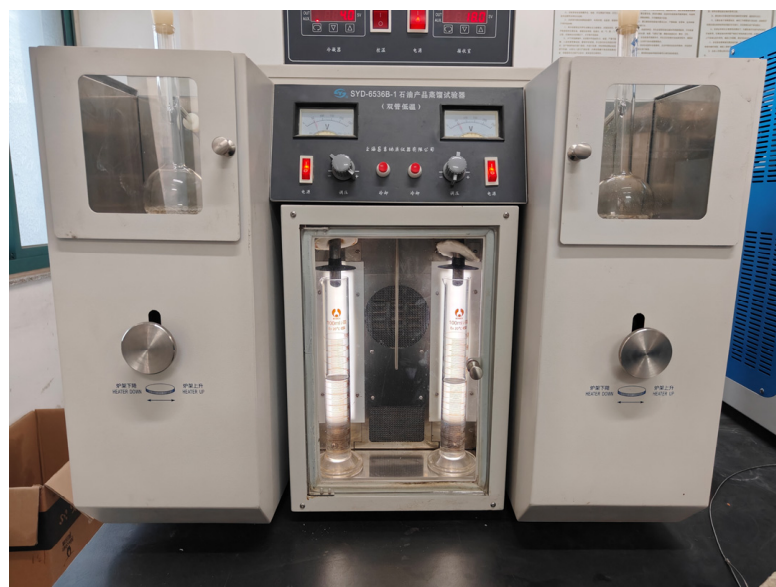
Figure 3. Experimental setup for measuring the distillation range of oil products. The Chinese characters marked on the equipment represent the official brand and model name of the experimental instrument.
