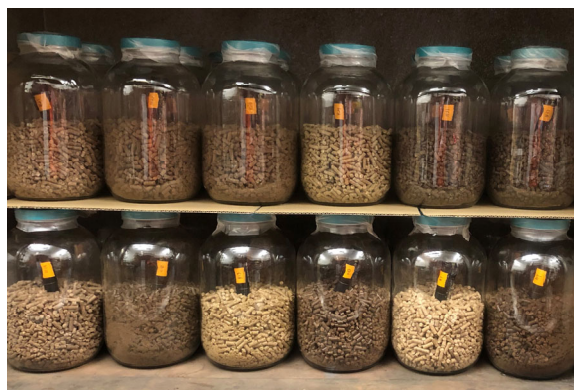
Figure 1. Carbon monoxide emissions experiment in a darkened laboratory hood under ambient conditions. Carbon monoxide sensors were placed in sealed, 3.84 L jars, and pellets were added until 50% headspace was achieved.
