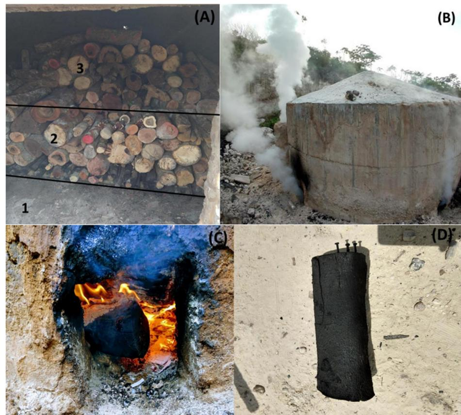
**Figure 2.** Carbonization process in a modified half-orange kiln. (A) Firewood arrangement: (1) first stacking, (2) second stacking, (3) third stacking; (B) firewood-to-charcoal transformation process; (C) blue smoke at the bottom of the kiln, indicating that carbonization is complete; (D) sample of recovered charcoal.
