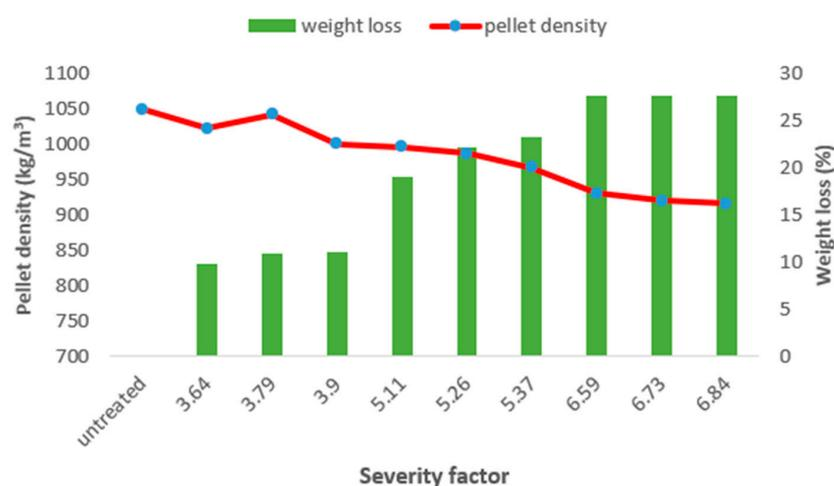
**Figure 7.** Pellet unit density and weight loss of raw WSS and WSS biochar for different severity factors.
