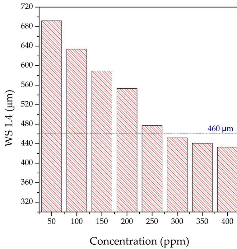
**Figure 2.** Impact of sunflower oil *N,N*-Bis(2-ethoxyethyl) amides addition on the lubrication characteristics of the base fuel.
