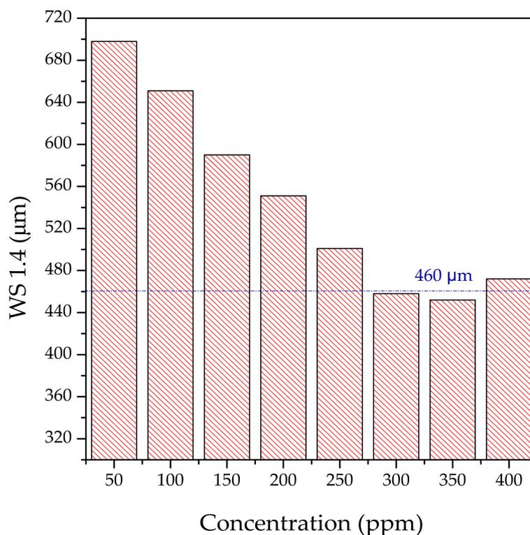
**Figure 8.** Impact of tobacco seed oil *N,N*-Bis(2-ethoxyethyl) amides addition on the lubrication characteristics of the base fuel.
