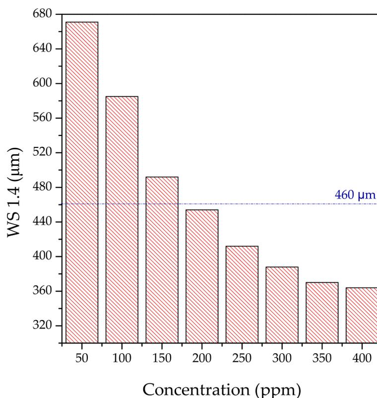
**Figure 4.** Impact of olive oil *N,N*-Bis(2-ethoxyethyl) amides addition on the lubrication characteristics of the base fuel.
