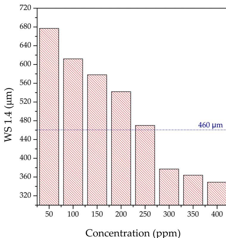
**Figure 5.** Impact of cottonseed oil *N,N*-Bis(2-ethoxyethyl) amides addition on the lubrication characteristics of the base fuel.
