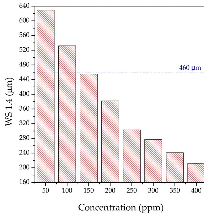
**Figure 6.** Impact of coconut oil *N,N*-Bis(2-ethoxyethyl) amides addition on the lubrication characteristics of the base fuel.
