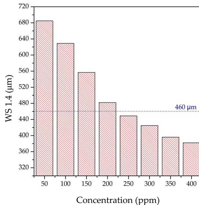
**Figure 7.** Impact of used frying oil *N,N*-Bis(2-ethoxyethyl) amides addition on the lubrication characteristics of the base fuel.
