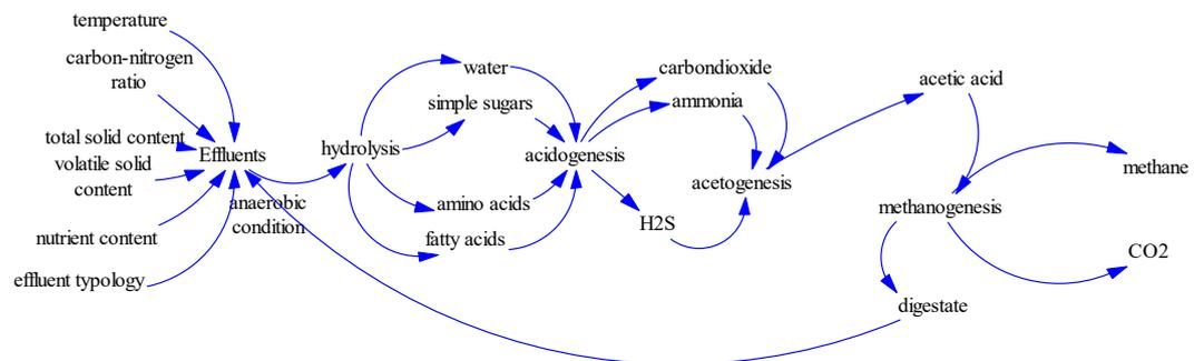
Figure 2. Adapted causal diagram of the anaerobic digestion of effluents used for biogas production [30].
