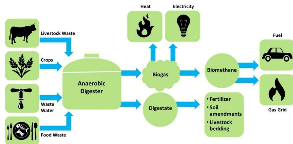
**Figure 1.** The material flow of the anaerobic digestion process and its uses [5].
