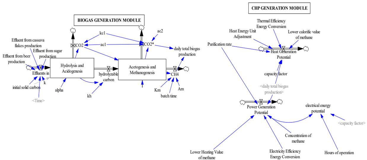
Figure 4. System dynamics biogas energy recovery model for CHP.
