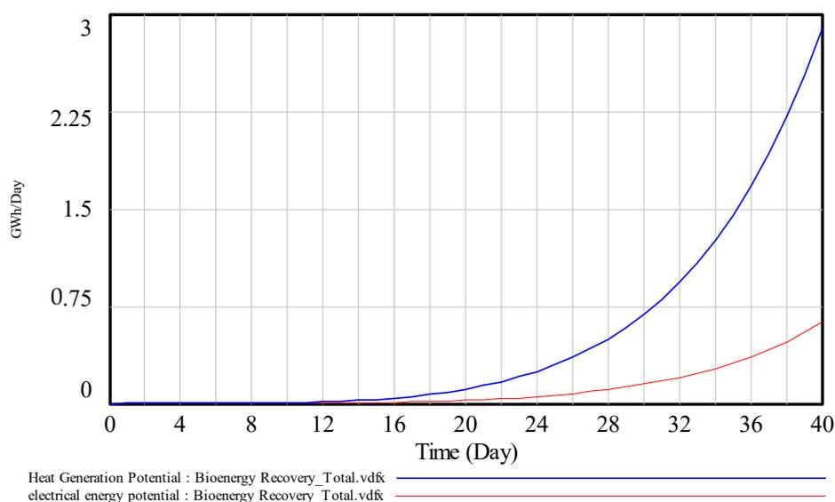
Figure 7. Heat and electrical energy potential from the biogas recovered from the effluents.
