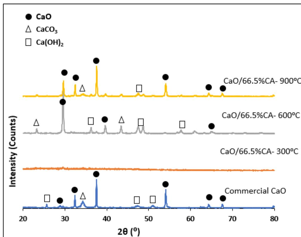
**Figure 4.** RXD pattern of CaO/CA and commercial CaO catalysts.
