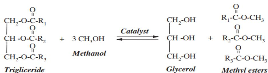
**Figure 1.** Transesterification reaction, where R<sub>1</sub>, R<sub>2</sub>, and R<sub>3</sub> are long hydrocarbon bonds.
