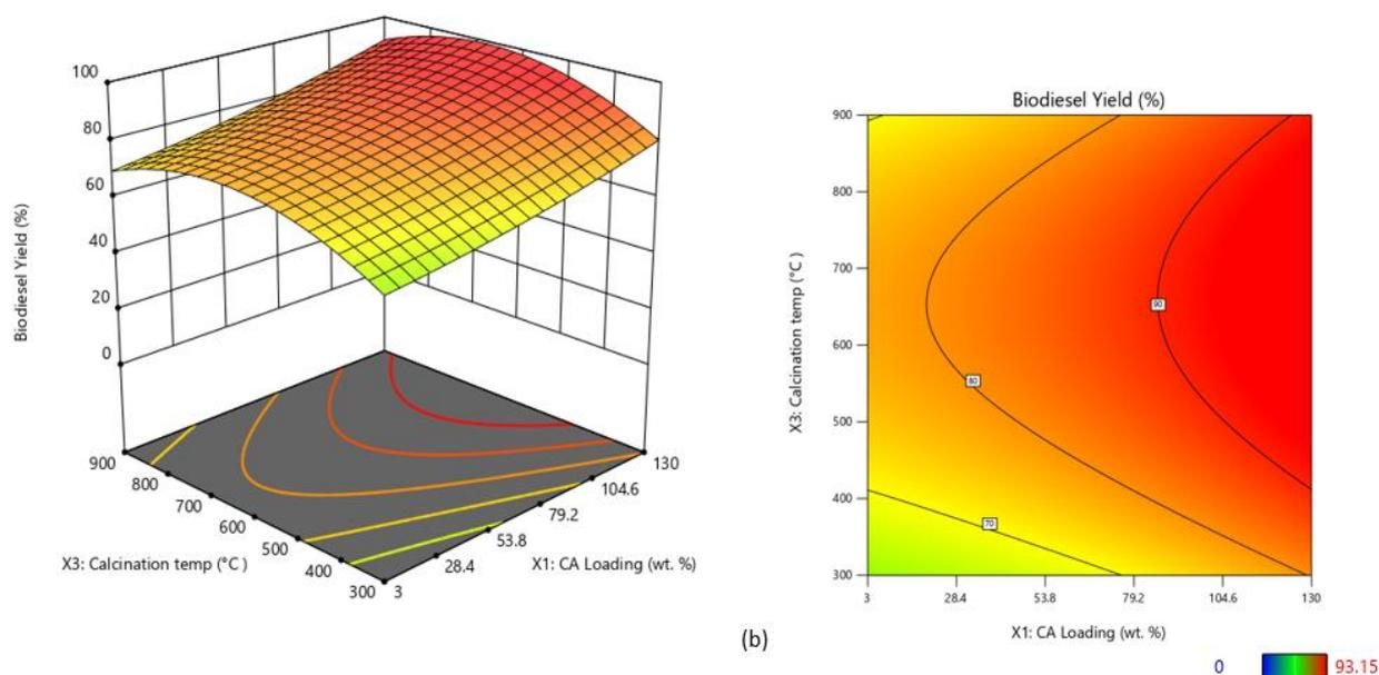
**Figure 10.** Three-dimensional surface and contour plots of biodiesel yield from the synthesized catalysts: (a) CaO/CA; (b) NaOH/CA.
