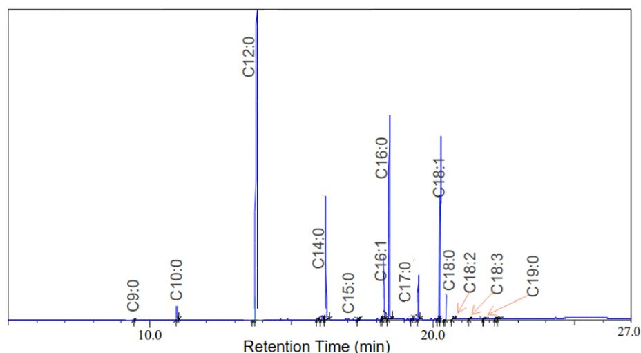
**Figure 11.** GCMS chromatographs of fatty acids and FAME derives from BSFL biodiesel.
