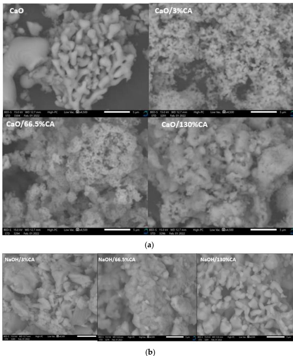
**Figure 3.** SEM micrographs of the catalysts with varied wt.% loading of citric acid: (a) CaO/CA catalysts; (b) NaOH/CA catalysts.
