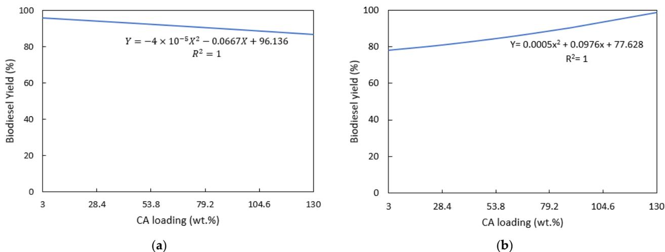
Figure 7. Effects of the citric acid loading wt.% on biodiesel yield: (a) CaO/CA; (b) NaOH/CA.
