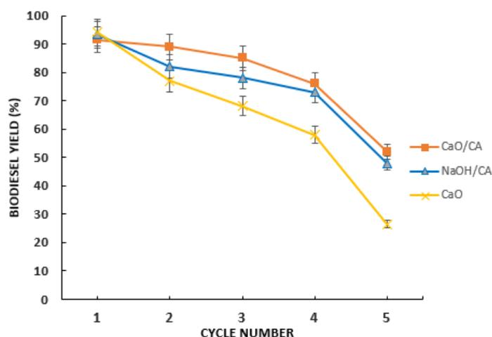
**Figure 13.** Biodiesel yield with different recycles of the catalyst in transesterification of BSFL oil.
