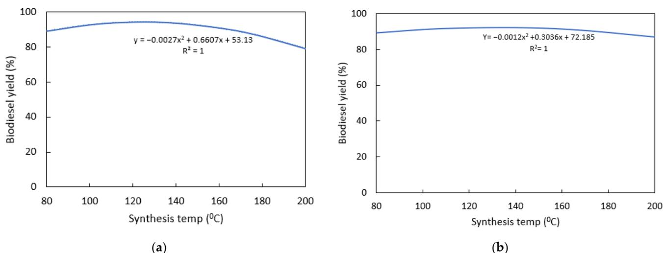
**Figure 8.** Effects of synthesis temperatures on biodiesel yield: (a) NaOH/CA; (b) CaO/CA.
