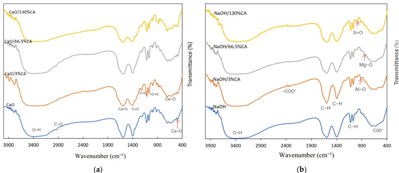
**Figure 2.** FTIR spectra of different CA loading wt.% on base catalyst: (a) CaO/CA; (b) NaOH/CA.
