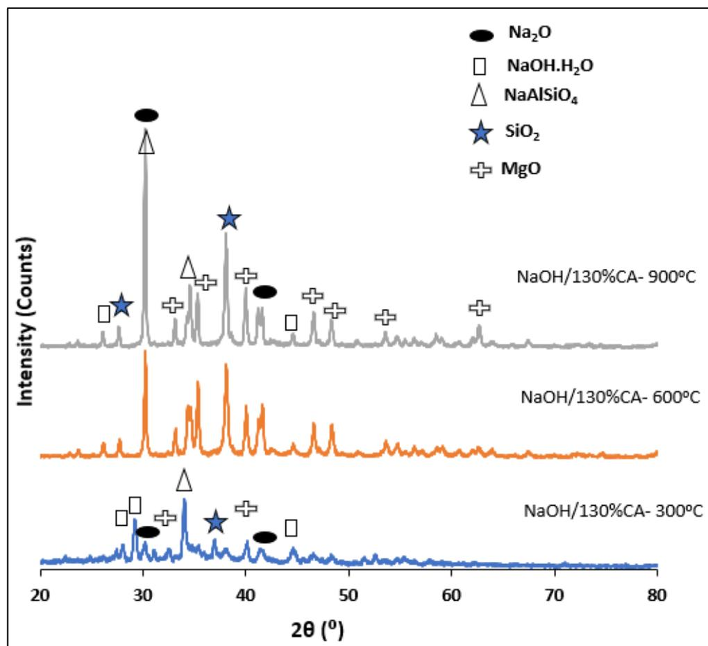
**Figure 5.** XRD pattern of NaOH/CA catalysts.
