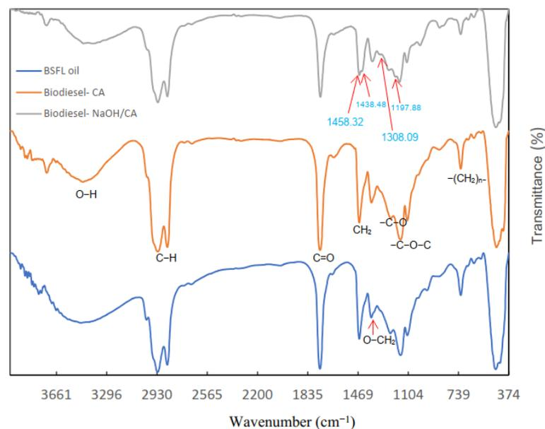
**Figure 12.** Comparison of FTIR spectra of BSFL-derived oil and biodiesel.
