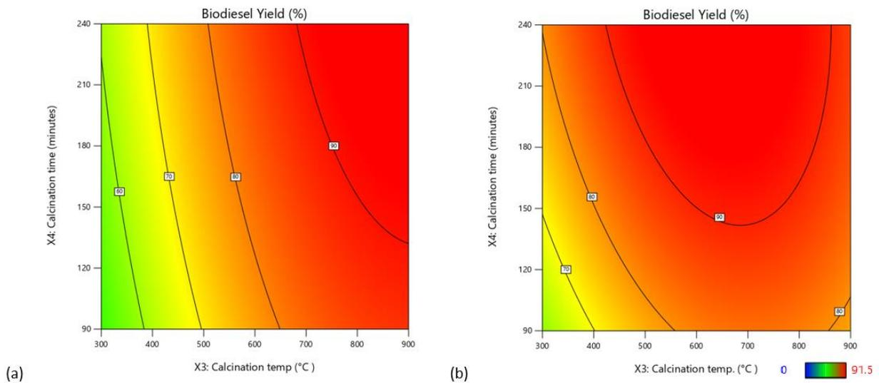
Figure 9. Effect of calcination temperatures and time on biodiesel yield: (a) CaO/CA; (b) NaOH/CA.
