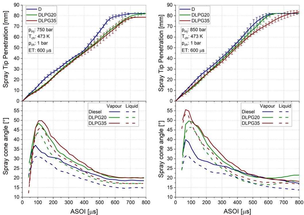
Figure 5. Spray characterization in terms of tip penetration and spray cone angle for different fuels under evaporating condition ( $T_{ch} = 473\text{ K}$ ).
