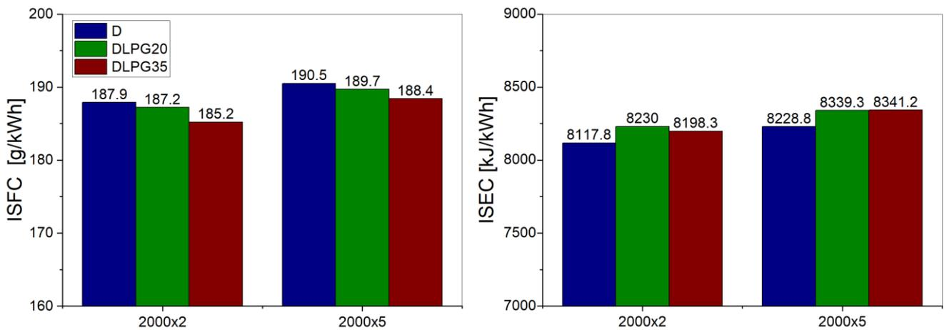
Figure 9. ISFC and ISEC parameters at 2000 r/min and different engine loads for the three blends.
