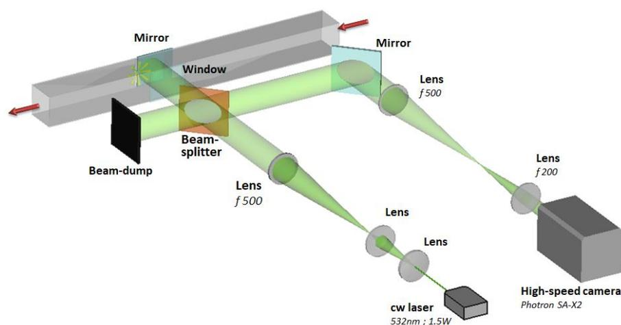
Figure 2. Optical setup.
