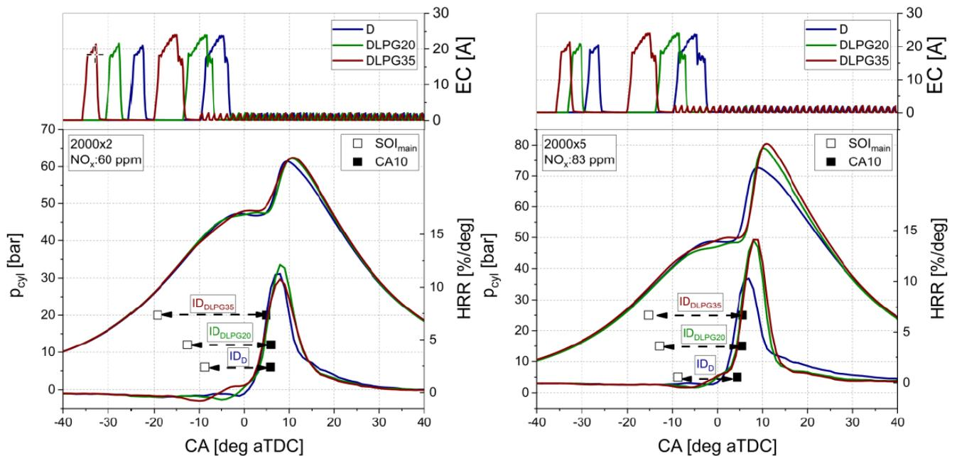
Figure 6. Pressure, HRR, Ignition Delay and injector energizing current at 2000 × 2 bar (left) and 2000 × 5 bar at constant NOx.
