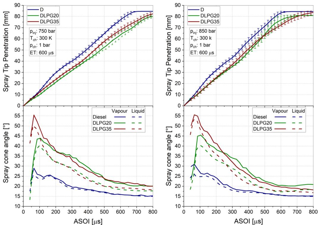
**Figure 3.** Spray characterization in terms of tip penetration and spray cone angle for different fuels under non-evaporation conditions ( $T_{ch} = 300$  K).
