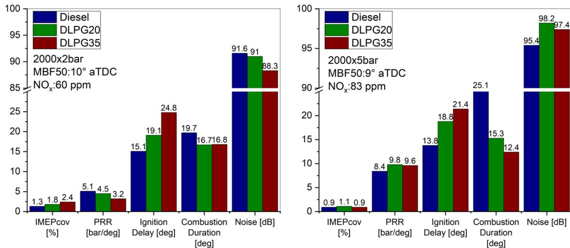
Figure 7. Combustion characteristics at 2000 r/min at different engine loads for different LPG-diesel blends compared to diesel.
