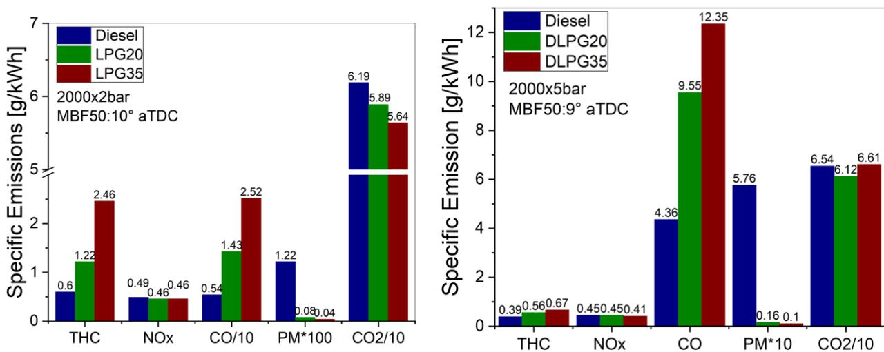
Figure 10. Emissions parameters at 2000 r/min and different engine loads for the three blends.
