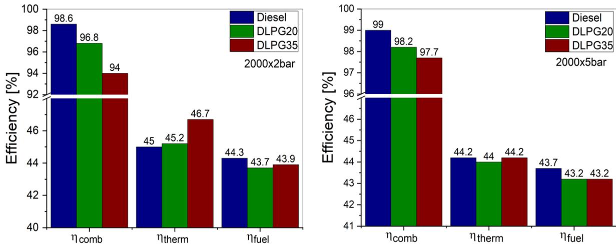
**Figure 8.** Efficiency parameters at 2000 rpm at different engine loads for different LPG-diesel blends compared to diesel.
