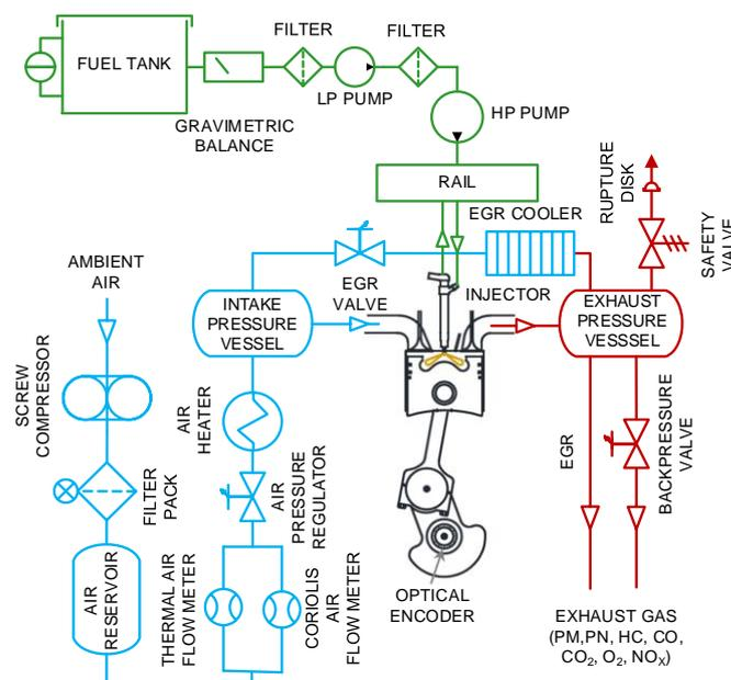
Figure 1. SCE test cell layout.
