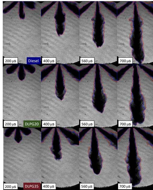
Figure 4. Spray sequence under evaporative conditions at rail pressure of 750 bar, liquid (blue), and vapor (red) detection for different fuels (diesel, DLPG20 and DLPG35).
