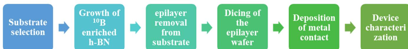
**Figure 2.** Schematic of h-BN detector fabrication process.
