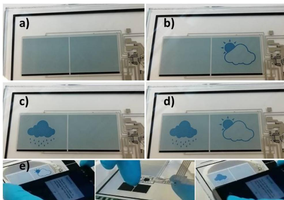
**Figure 4.** (a–d) Photographs showing the different coloration states of the screen printed electrochromic display; (e) The photographs describe a demonstration sequence of the system, where the batteryless hybrid printed electronic sensor platform is activated by energy harvesting through the NFC interface of a mobile phone. (Left) A dry sensor state is visualized on the display. (Middle) A water drop is placed on the sensor area. (Right) A wet sensor state is visualized on the display.
