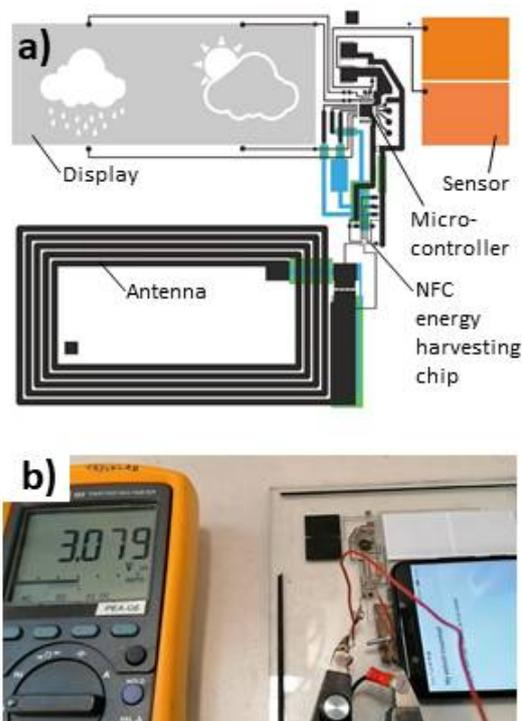
**Figure 1.** (a) Schematic showing a few of the screen printed layers: the first silver layer (black), the insulating layer defining the electrochromic “rain” and “sun” display segments (gray), the carbon electrodes of the sensor (orange), the insulating layer required to prevent short-circuits (green), and the second silver layer to establish wire crossings (blue); (b) The continuous voltage output level upon activating the system through the NFC interface of a mobile phone.
