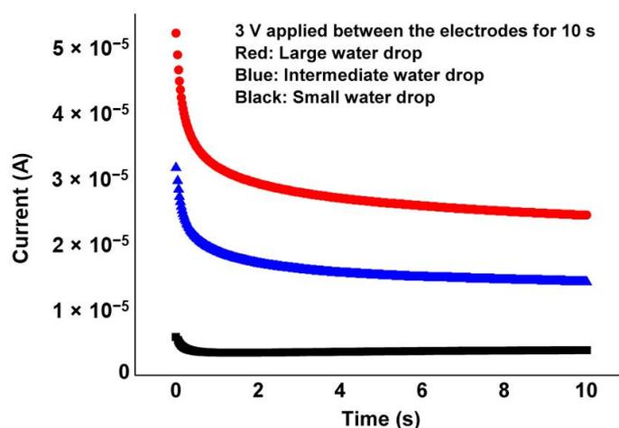
**Figure 2.** Water droplets of three different volumes, thereby creating three different interface areas between the water and the carbon-based sensor electrodes, result in different current vs. time characteristics. The volumes of the three water droplets denoted small, intermediate and large correspond to approximately 100, 500 and 1000  $\mu\text{L}$ , respectively.
