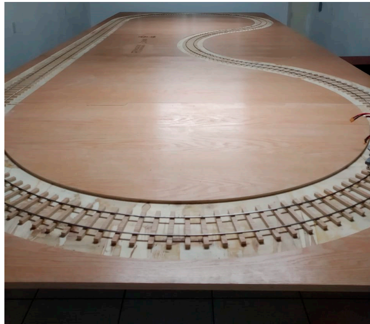
Figure 2. Panoramic view of the testbed. The rails are a \beta -shaped closed loop track.
