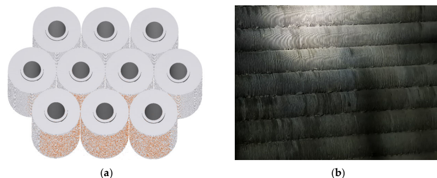
Figure 3. Comparison between simulated and experimental results of dust deposition: (a) Simulated dust deposition pattern; (b) Experimental fouling distribution.
