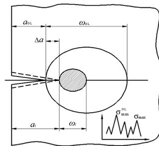
**Figure 1.** The diagram of Willenborg–Chang crack model with a random load spectrum. The crack with full lines is the old crack with a length of  $a_{OL}$ , and the dash line crack is a new one with a length of  $a_{OL} + \Delta a$ .
