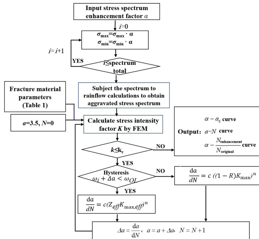
Figure 2. Flow chart of random load spectrum crack growth enforcement calculation program.
