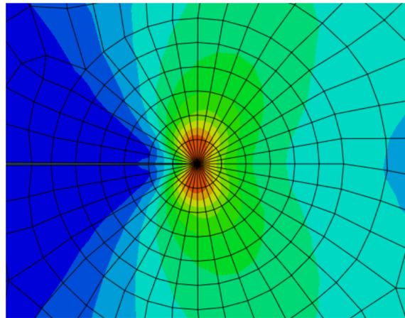
Figure 4. Crack tip finite element stress.
