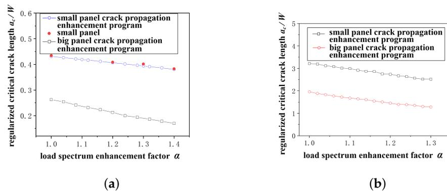
**Figure 9.** (a) Constant amplitude spectrum enhanced regularized  $\alpha - a_c$  curve. (b) Random amplitude spectrum enhanced regularized  $\alpha - a_c$  curve.
