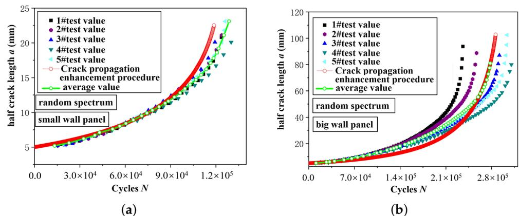
**Figure 6.** (a) Load spectrum  $a - N$  curve of small wall panel. (b) Load spectrum  $a - N$  curve of big wall panel.
