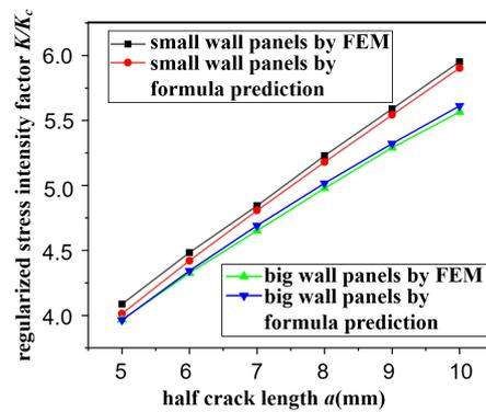
Figure 7.  $a - K$  curve with different calculation methods.
