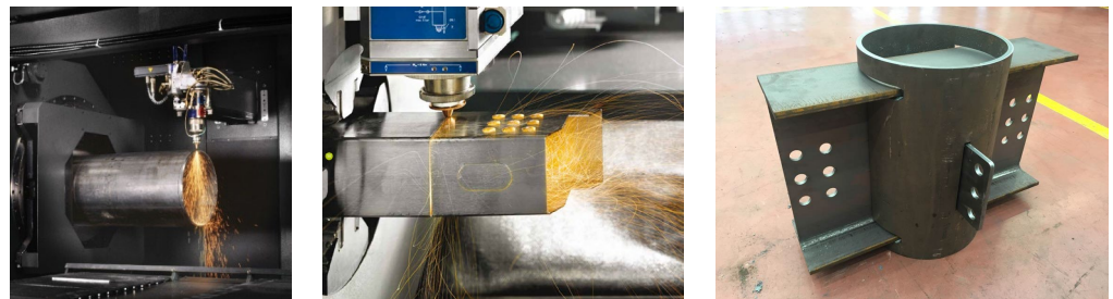
Figure 2. Examples of the laser cutting process and a four-way LASTEICON joint [30].
