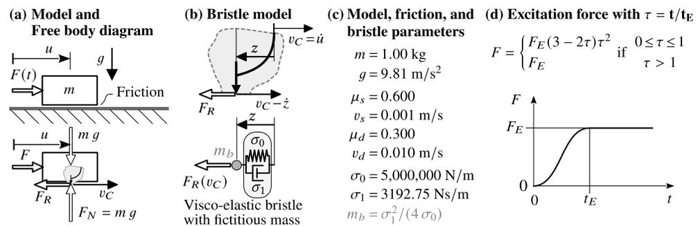
Figure 2. Virtual friction test-bench.
