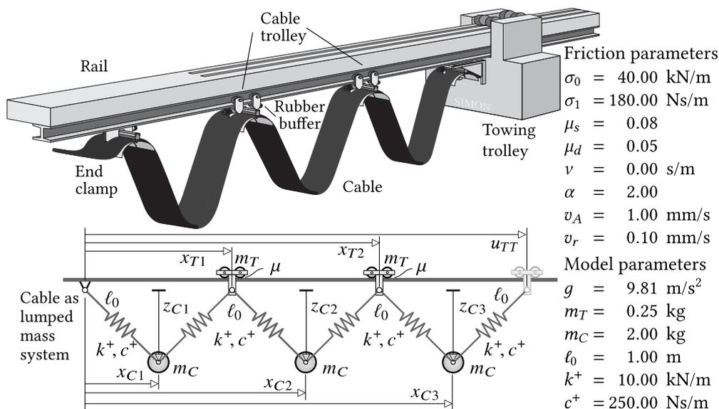
Figure 10. Multibody model of a crane festoon system as defined in [4].
