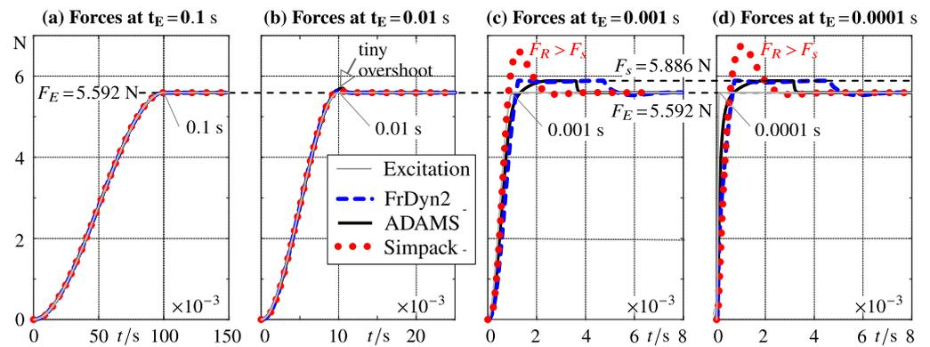
**Figure 6.** Dynamic friction forces resulting from step force excitation with different durations.
