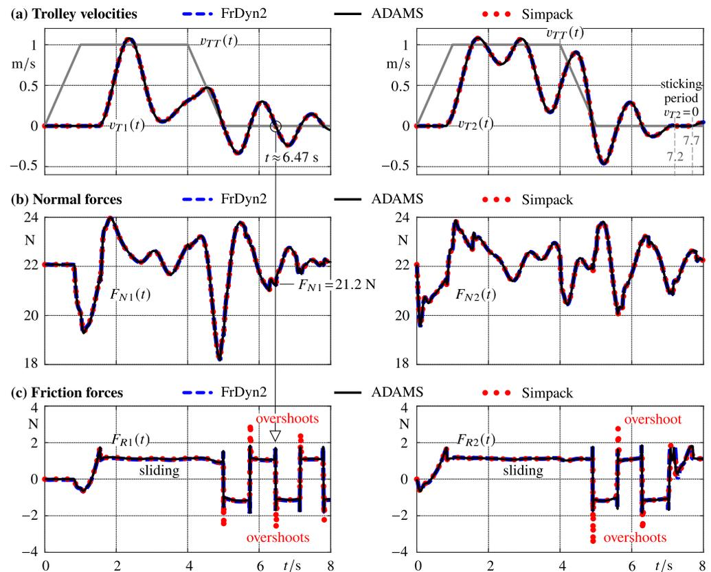
**Figure 11.** Results of a simulated festoon extension maneuver.
