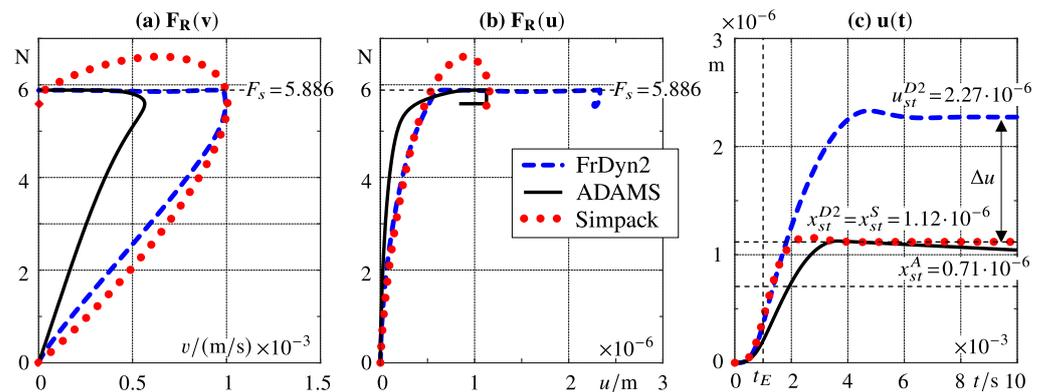
**Figure 8.** Friction force characteristics and body displacements at a step duration of  $t_E = 0.001 \text{ s}$ .
