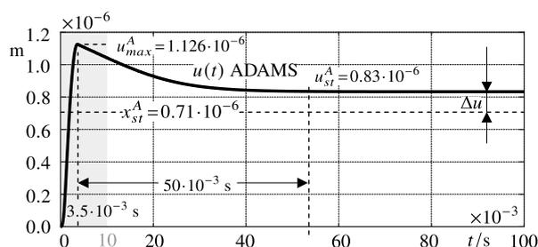
Figure 9. Body displacements generated with Adams at a step duration of  $t_E = 0.001$  s.
