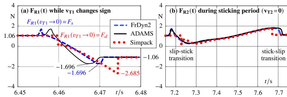
Figure 12. Friction forces in specific time intervals.
