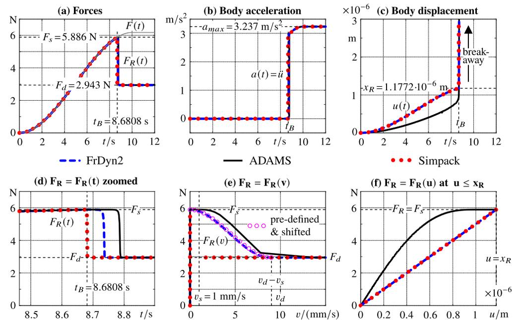
Figure 5. Virtual friction test-bench simulation results with a force that exceeds the adhesion limit.
