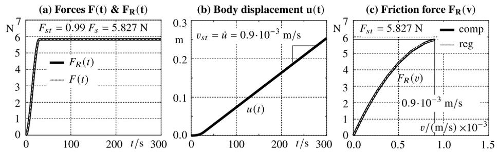
Figure 4. Slow sliding approximates sticking at a standard static friction model.
