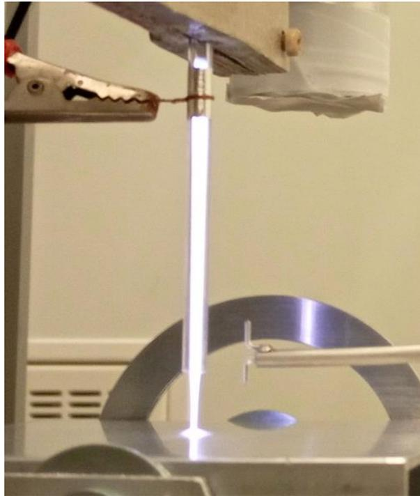
**Figure 8.** A typical configuration of the dipole antenna to detect the plasma discharge signal: measuring the electromagnetic field irradiated by the plasma.
