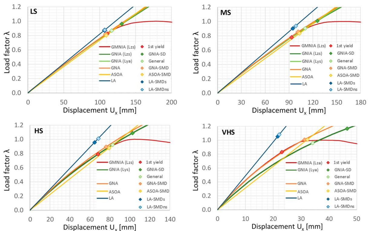
**Figure 12.** Comparison between the equilibrium paths of the examined frames marked with the point corresponds to collapse.
