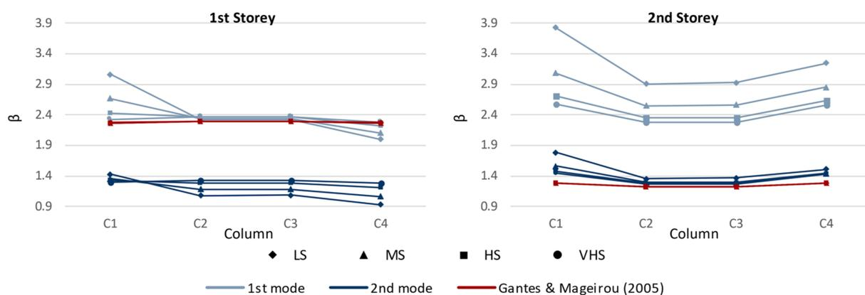
Figure 18. Comparison between effective lengths calculated with different approaches.
