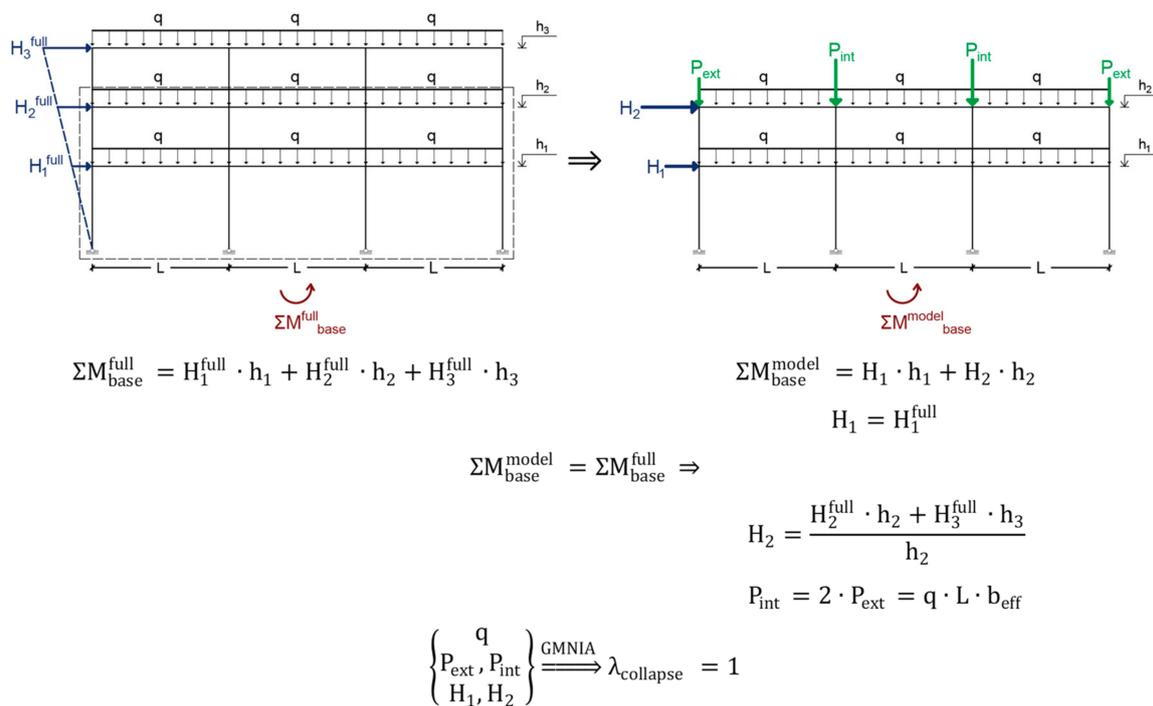
Figure 4. Derivation of loads for the examined frames (MS).
