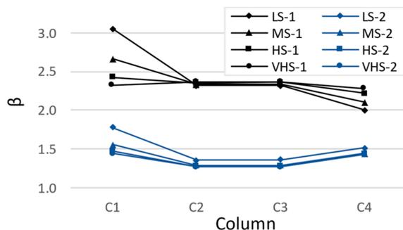
**Figure 16.** Buckling length factors determined from the 1st sway buckling mode for the 1st floor columns and the 2nd sway buckling mode for the 2nd floor columns.
