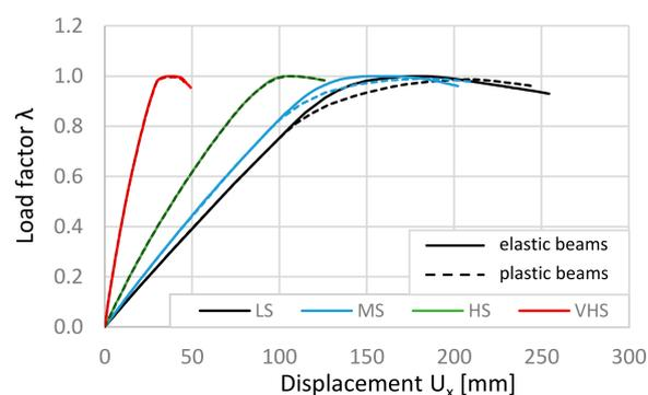
**Figure 6.** Comparison of the behaviour of the frames considering elastic and elastoplastic beams.
