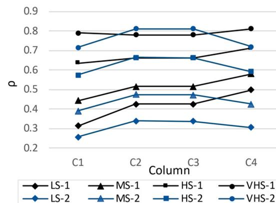
**Figure 17.** Strut indexes of the examined columns.
