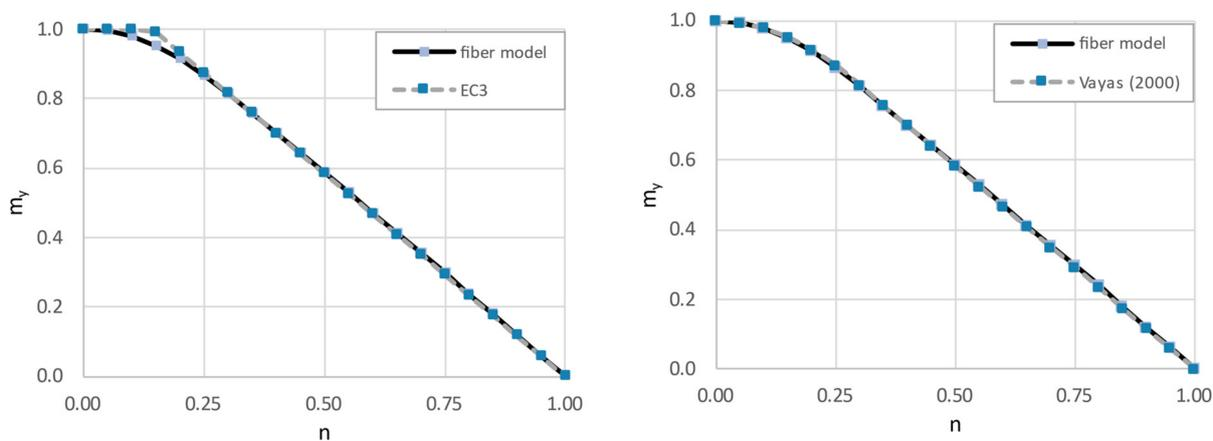
Figure 2. Comparison of interaction resistance diagrams  $n + m_y$  of numerical analysis (fiber model) and analytic formulae EC3 [1], Vayas (2000) [26] for a HEB 450 section.
