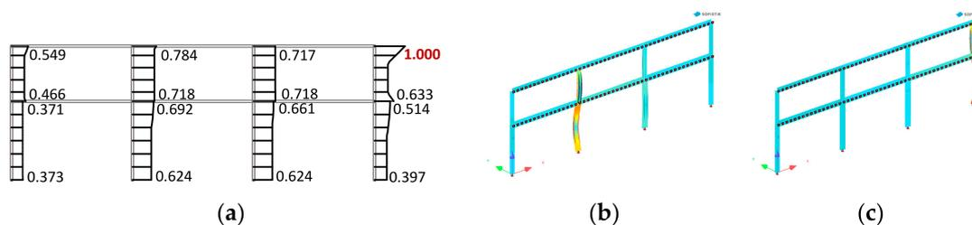
**Figure 14.** Implementation of the General method on the VHS frame: (a) utilization of the columns for the determination of  $\alpha_{util,k}$ ; (b) first out-of-plane buckling mode of the frame; (c) first out-of-plane buckling mode that includes the most stressed column.
