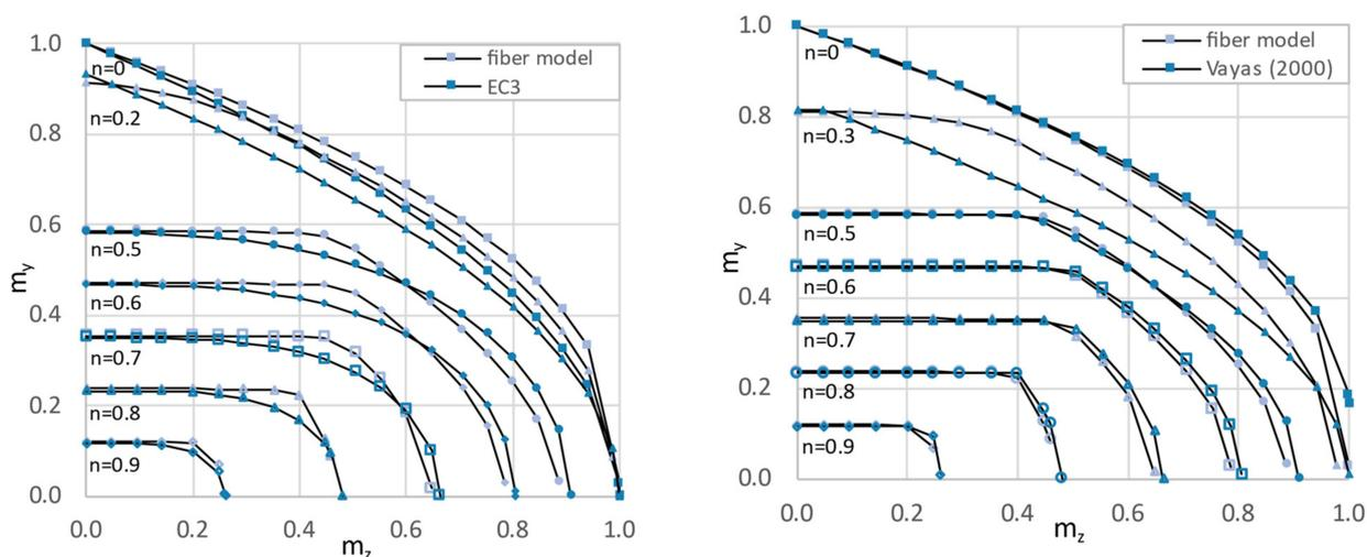
Figure 1. Comparison of interaction resistance diagrams  $n + m_y + m_z$  of numerical analysis (fiber model) and analytic formulae EC3 [1], Vayas (2000) [26] for a HEB 450 section.
