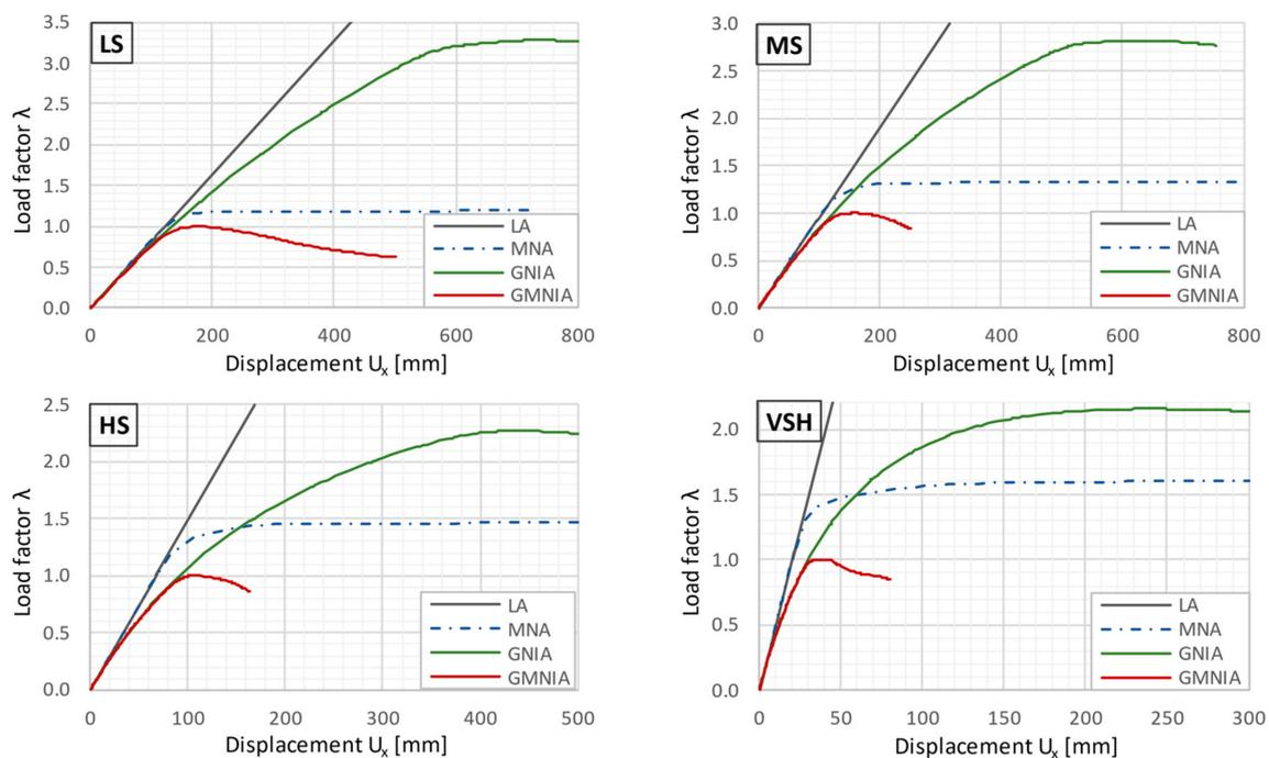
**Figure 7.** Equilibrium paths of the examined frames as derived with different methods of analysis.
