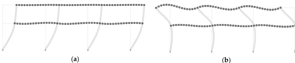
**Figure 15.** Two first in-plane sway buckling modes of the examined frames. (a)—1st sway buckling mode; (b)—2nd sway buckling mode.
