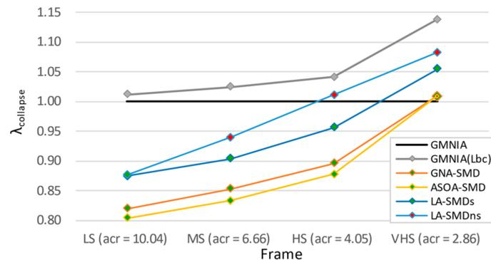
**Figure 13.** Comparison of the ultimate load factors of the methods that involve buckling verifications with those of GMNI Analyses taking into account local imperfections either from Table 5.1 of EN 1993-1-1 [1] or from the Equation (12).
