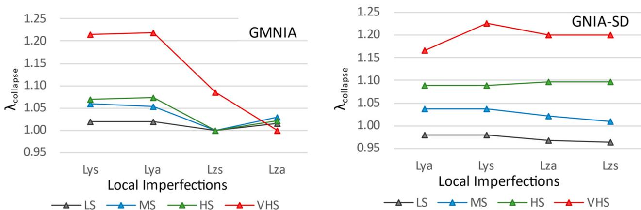
**Figure 8.** Variation of the ultimate load factor with the imperfection pattern for GMNIA and GNIA-SD methods.
