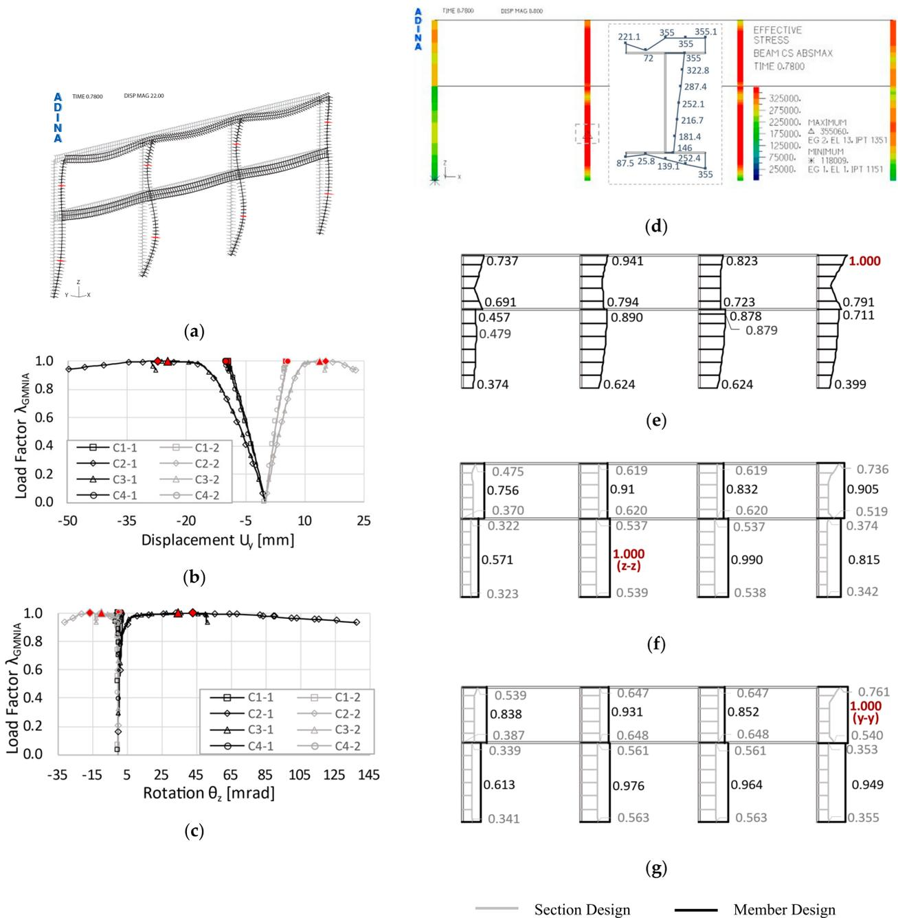
**Figure 10.** Collapse mechanism and utilization level of VHS frame—(a) deformed shape (GMNIA); (b,c) equilibrium paths (GMNIA); (d) stress distribution (GMNIA); (e) utilization level (GNIA-SD); (f) utilization level (GNA-SMD); (g) utilization level (LA-SMDs).
