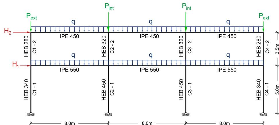
**Figure 3.** Configuration and load pattern of the examined frames and designation of their columns.
