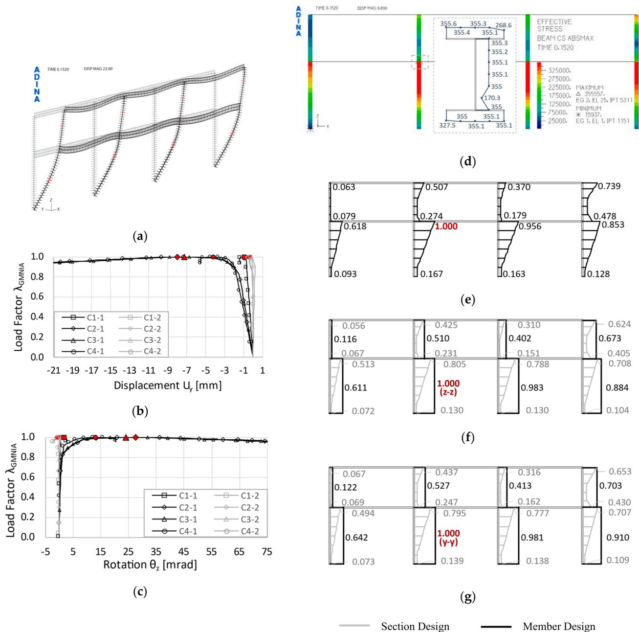
**Figure 9.** Collapse mechanism and utilization level of LS frame—(a) deformed shape (GMNIA); (b,c) equilibrium paths (GMNIA); (d) stress distribution (GMNIA); (e) utilization level (GNIA-SD); (f) utilization level (GNA-SMD); (g) utilization level (LA-SMDs).
