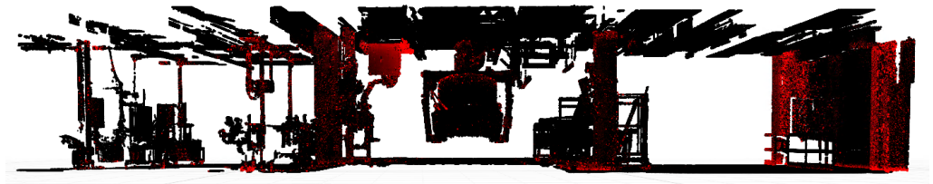
Figure 5. Visualization of an assembly tact of the test set, where certain predictions are displayed in black and uncertain predictions are displayed in red. In this case, the network (un)certainty is evaluated by using the method based on credible interval estimation.
