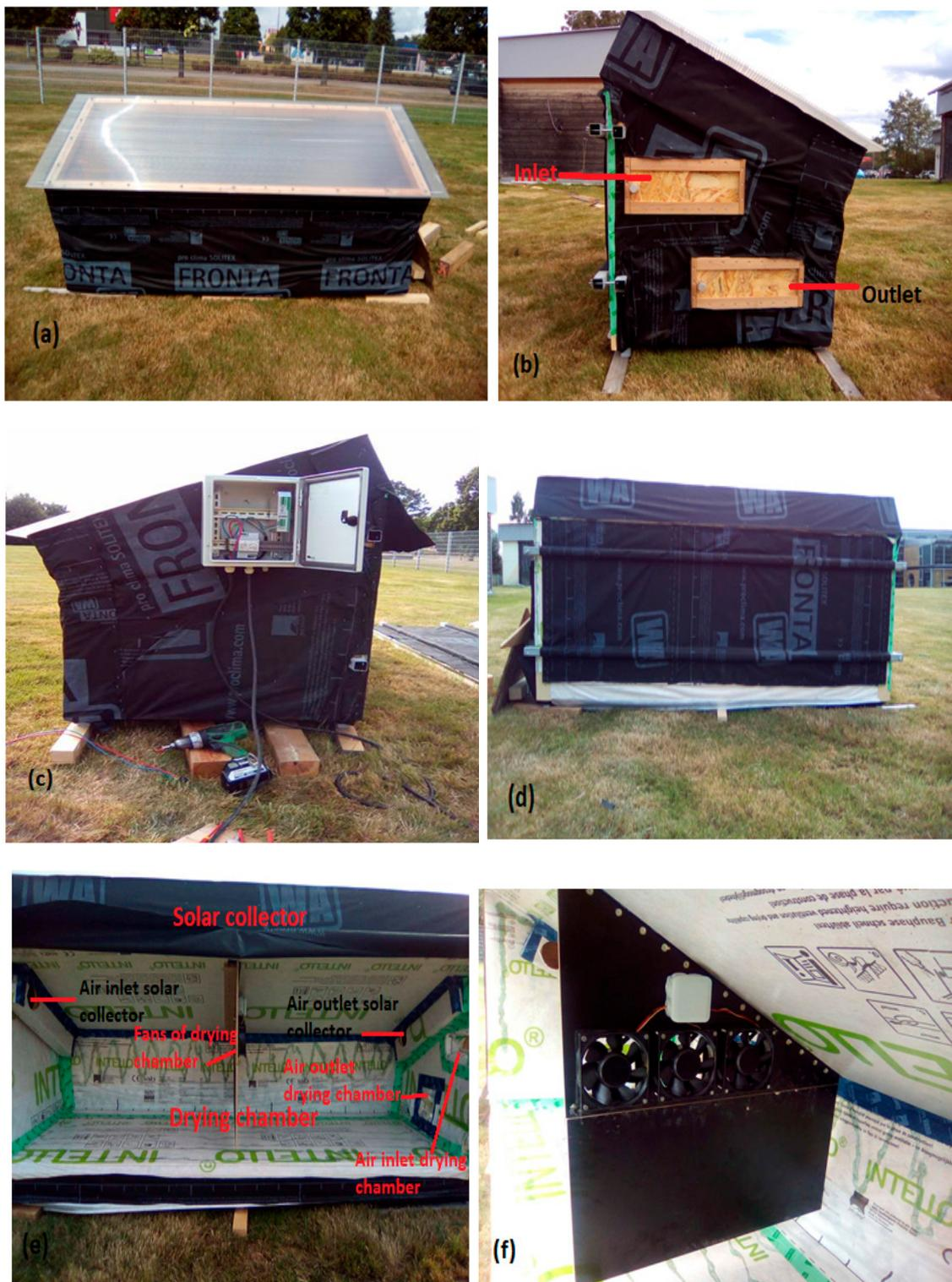
**Figure 1.** Presentation of the studied solar dryer, (a) south side and solar collector, (b) west side modular openings, (c) east side and electrical cabinet, (d) north side and door, (e) drying chamber, (f) fans in the drying chamber.
