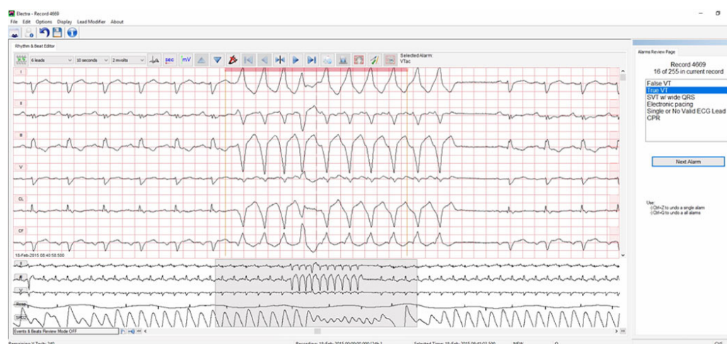
Figure 6. Illustrates an arrhythmia alarm for ventricular tachycardia ready for annotation using the Continuous ECG Recording Suite (CER-S) software program. The annotator selected a response (true, false, etc.) and then selected “Next Alarm” to move onto the next annotation. Note that an SpO2 waveform is shown in the bottom context view for use by the annotator when making a decision. Arterial blood pressure is also available if the patient has this device in place. Figure from the Center for Physiologic Research, UCSF School of Nursing.
