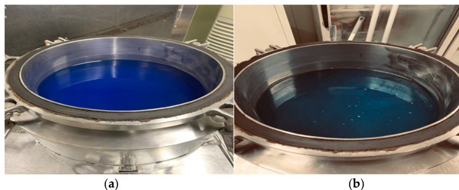
Figure 5. The manufactured vanadium electrolyte ( 3.5^+ ) in 20 L hydrothermal reactor. (a): vanadium ( 4^+ ) electrolyte reduced using citric acid. (b): manufactured vanadium ( 3.5^+ ) electrolyte by HRR.
