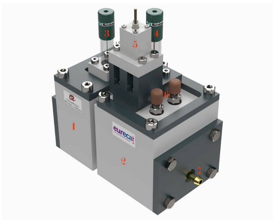
Figure S1. 3D rendered design of Teflon H-cell used for the experiments.
