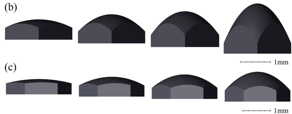
Figure 7. The microlenses demolded from the molds with radius of 1 mm and \alpha of 10^\circ , 20^\circ , 30^\circ , and 40^\circ , respectively. (a) The round microlenses. (b) The square microlenses. (c) The hexagonal microlenses.
