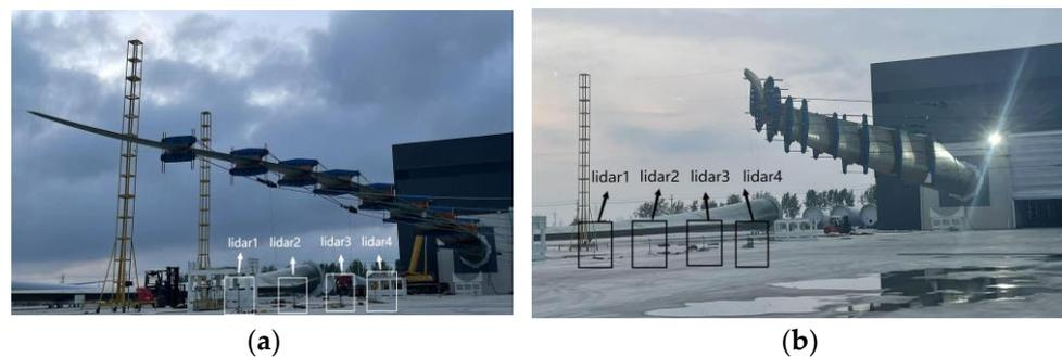
**Figure 2.** Static loading test scene. (a) Minimum oscillation direction, (b) maximum swing direction.
