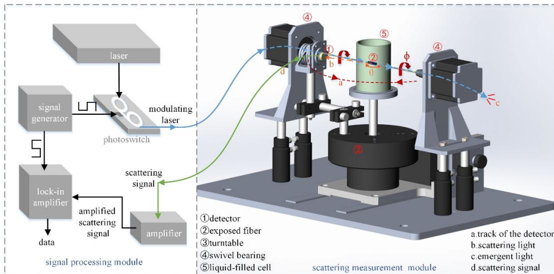
**Figure 3.** Fiber scattering measurement equipment.
