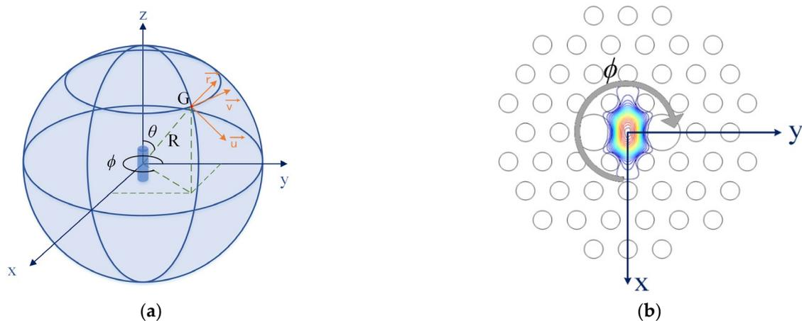
**Figure 1.** (a) Illustration of scattering of point G on a distant sphere and (b) the scattering simulation model of the solid-core PM-PCF.
