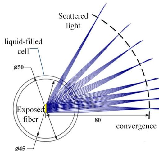
**Figure 4.** Simulation of convergence position of scattered light.
