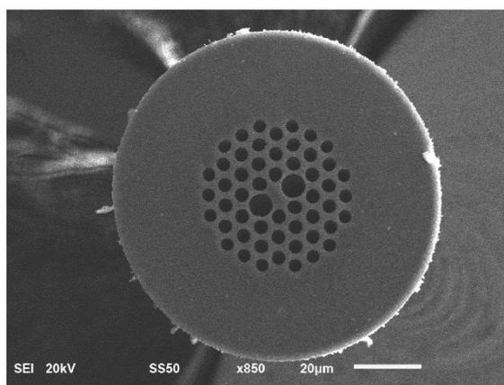
Figure 5. A section of PM-PCF for gyroscopes.
