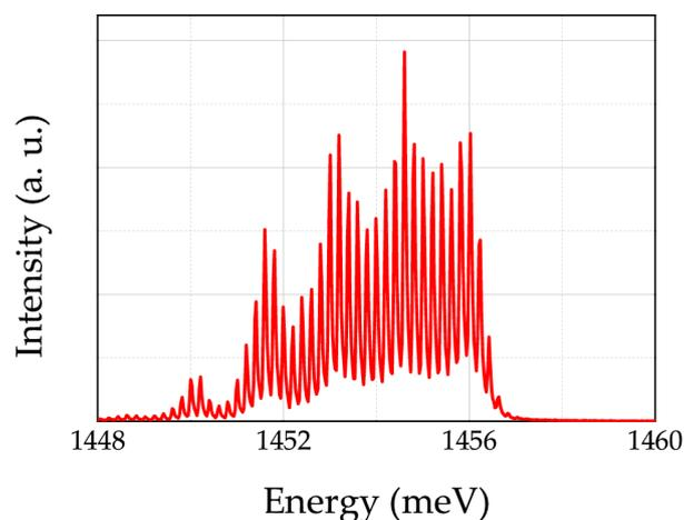
**Figure 1.** Optical spectrum of the multimode semiconductor Fabry-Perot (FP) laser.
