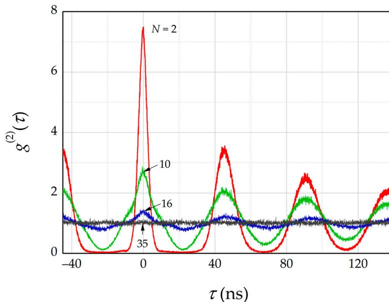
**Figure 2.** The intensity correlation functions  $g^{(2)}$  obtained by an ordinary Hanbury Brown and Twiss (HBT) setup.  $N$  is the number of simultaneously detected longitudinal modes shown in Figure 1.
