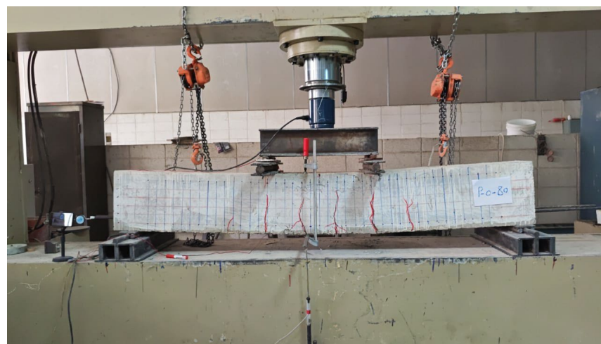
Figure 7. Typical flexural failure and concrete crushing observed in tested bridge girder specimens.
