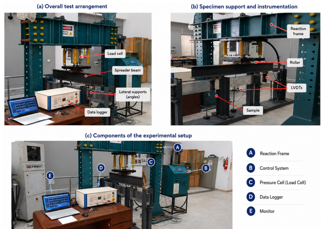
Figure 4. Experimental setup for four-point bending tests: (a) overall test arrangement; (b) specimen support and instrumentation; and (c) components of the loading and data acquisition system.
