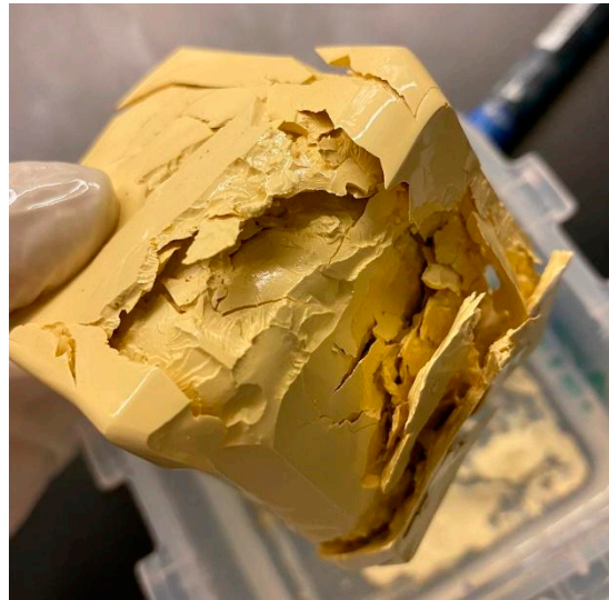
Figure 11. Novel Cement Sample After Placement in Acetone for 10 Consecutive Days.
