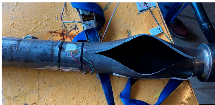
Figure A5. Schedule 80 Pipe 1 after bursting.
