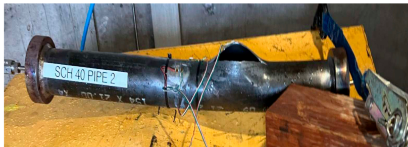
Figure A4. Schedule 40 Pipe 2 after bursting.
