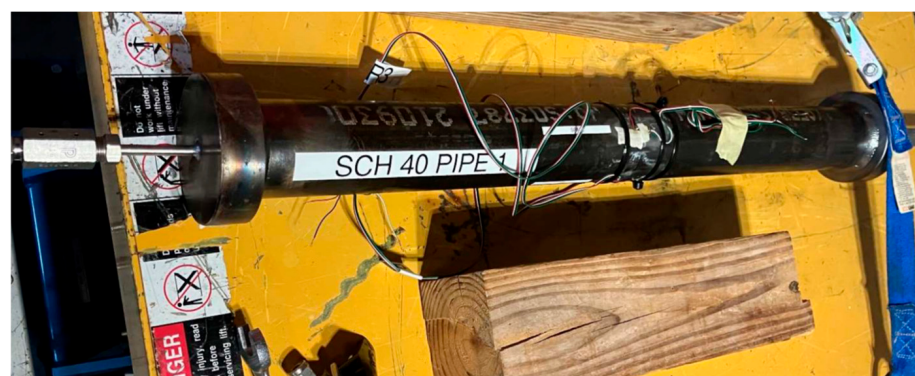
Figure 6. Pressure burst test setup for SCH-40 Pipe 1.
