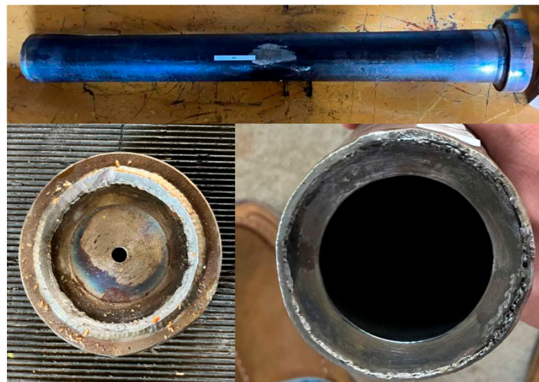
Figure A7. Schedule 160 Pipe 2 after bursting.
