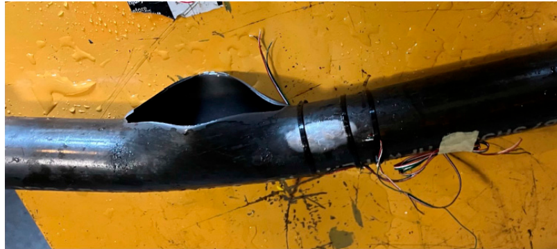
Figure A3. Schedule 40 Pipe 1 after bursting.
