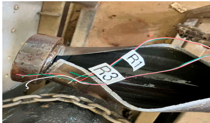
Figure A6. Schedule 80 Pipe 2 after bursting.
