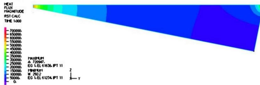
Figure 4. Heat flux distribution within the film for a typical period.
