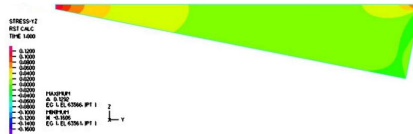
Figure 8. Shear stress distribution on the lower surface of the droplet.
