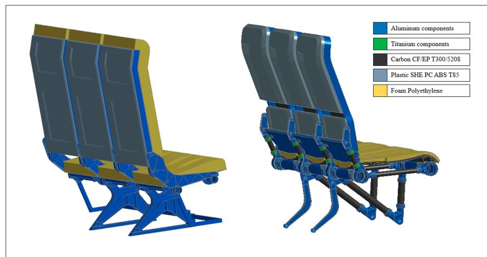
Figure 5. Material usage in the initial version (left) and improved version (right).
