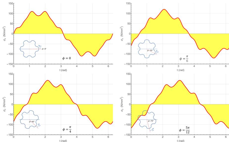
Figure 10. Distribution of the bending stresses on the M-T04 profile for several rotation angles according to Equation (52).
