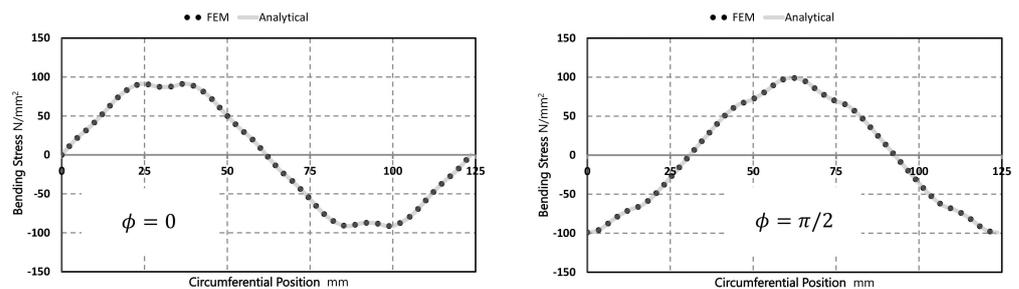
Figure 12. Distribution of the bending stresses on the M-T04 profile for two rotation angles: FEM results and analytical solution based on Equation (55).
