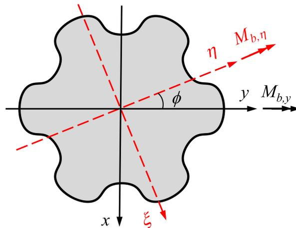
Figure 6. Rotated coordinate system for the profile cross-section.
