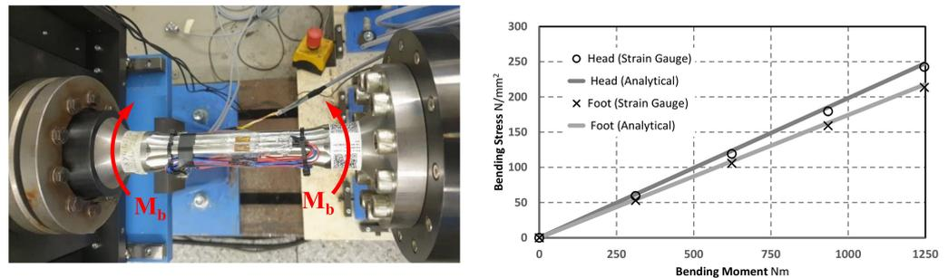
**Figure 13.** Testbench for the bending load, with a strain-gauge application (left); comparison of the analytical solution of Equation (55) with the experimental data (right) [2].
