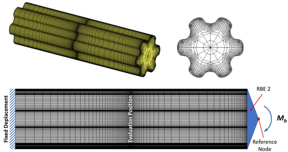
Figure 8. FE mesh and boundary conditions for the M-T04 profile.
