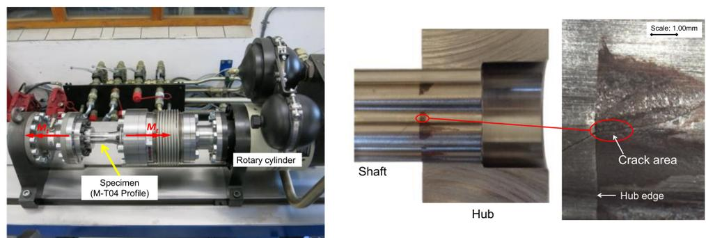
**Figure 4.** Testbench for the torsional load (left) and the cracking due to torsional loading (right) [1].
