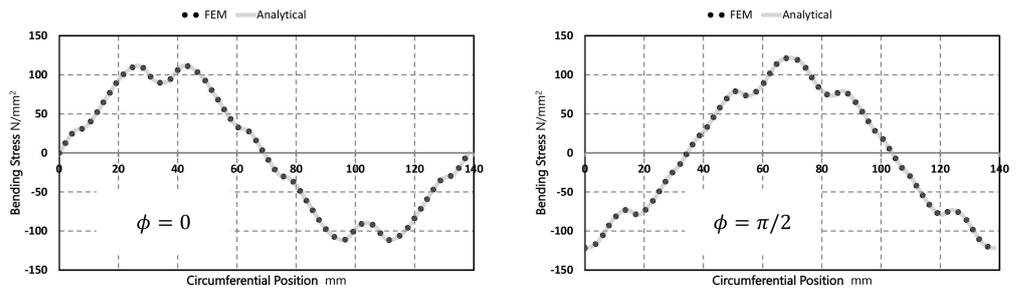
Figure 9. Distribution of the bending stresses on the M-T04 profile for two rotation angles: FEM results and analytical solution based on Equation (52).
