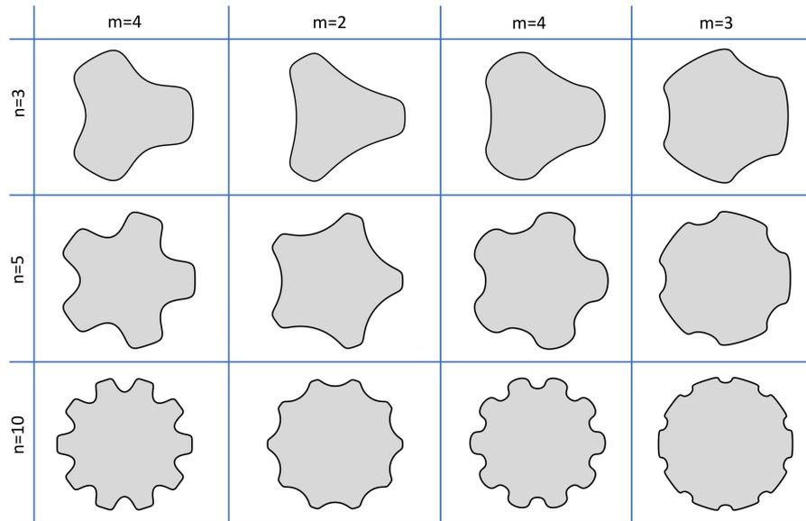
**Figure 2.** Examples of the complex hybrid trochoid (M-profiles) with additional eccentricities, where  $m$  represents the order and  $n$  represents the periodicity of the profile.
