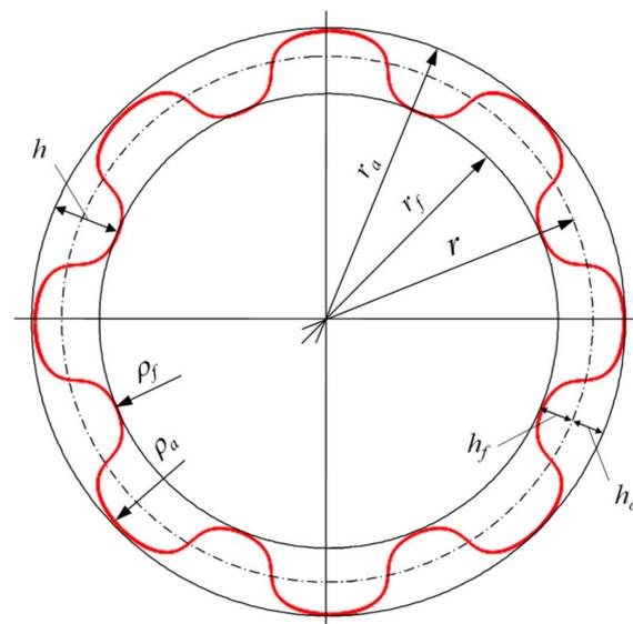
**Figure 3.** Geometry of the M-T04 family for  $n = 8$  (exemplary) [1].
