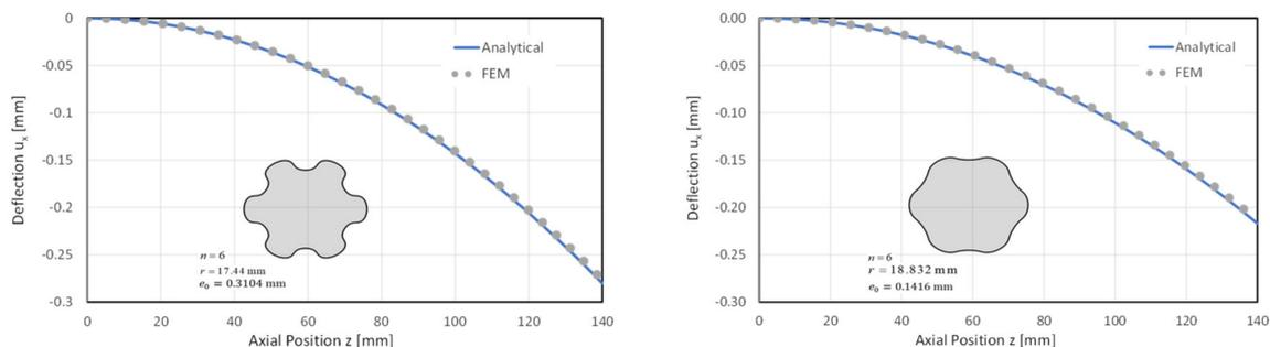
**Figure 14.** Shaft deflection of the M-04 [1] (left) and the modified profile [2] (right): comparison between the FE analysis results and the results based on Equation (36c).
