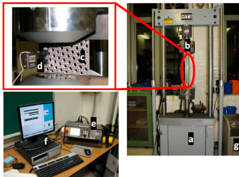
Figure 11. Experimental set-up and instrumentation. (a) 100 KN MTS machine (b) load cell (c) mounted test specimen (d) 632-31E-24 extensometer (e) DAQ (f) monitoring software (g) MTS 685 hydraulic controller.
