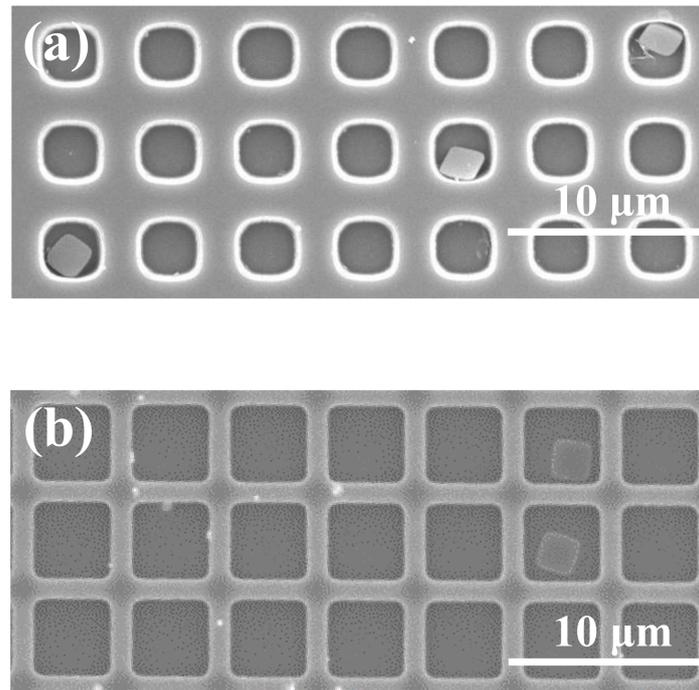
Figure 5. Typical plane-view scanning electron microscope images of (a) the SiO<sub>2</sub>-terrace receiver and (b) the reference receiver.
