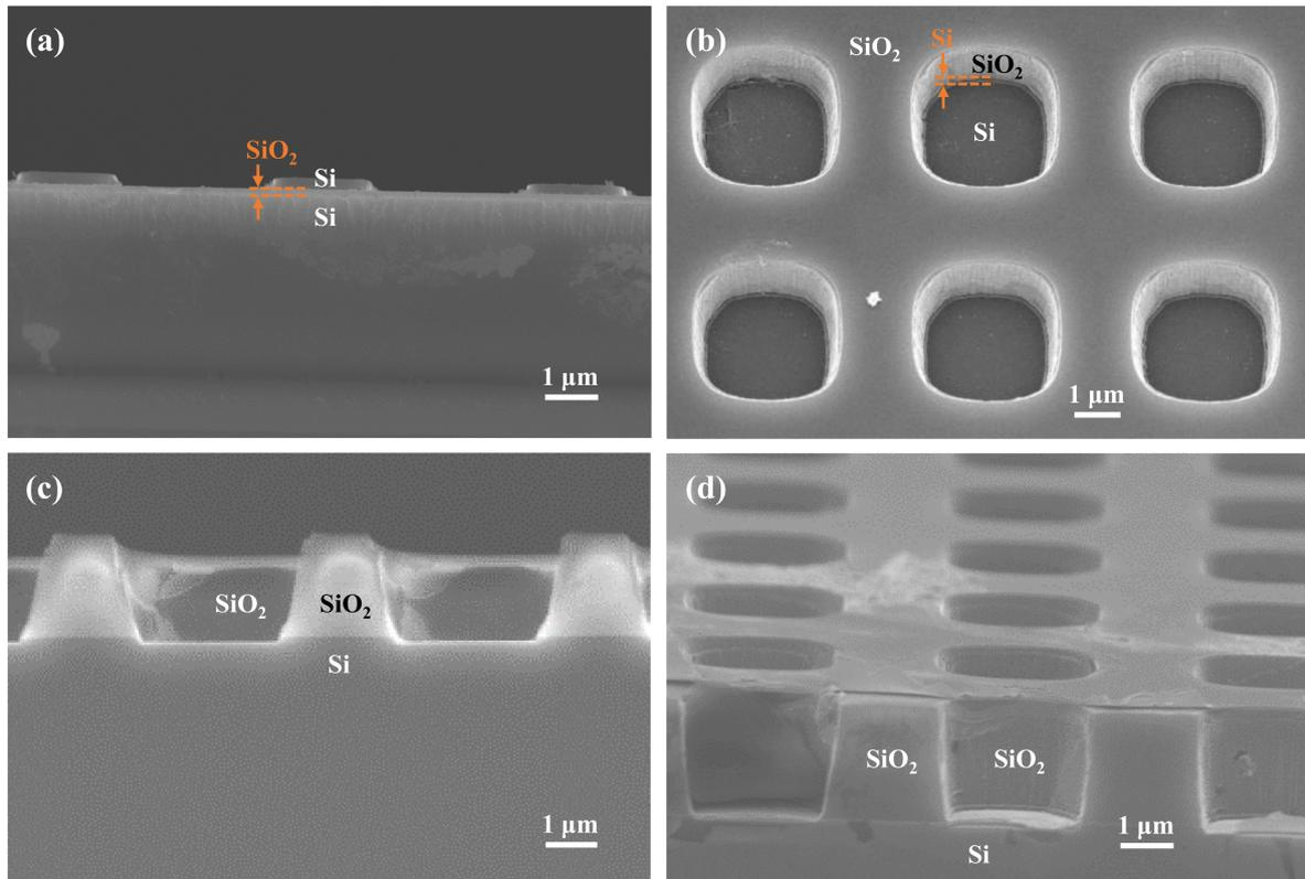
**Figure 3.** (a) Cross-sectional scanning electron microscope image of the releaser piece, (b) bird’s-eye-view and (c) cross-sectional scanning electron microscope images of the receiver piece with an SiO<sub>2</sub> terrace before the submergence process, and (d) bird’s-eye-view scanning electron microscope image of the receiver piece with an SiO<sub>2</sub> terrace after the submergence process.
