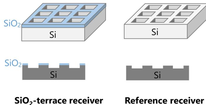
**Figure 4.** Schematic bird’s-eye views and cross-sectional views of the SiO<sub>2</sub>-terrace receiver and the reference Si-only receiver.
