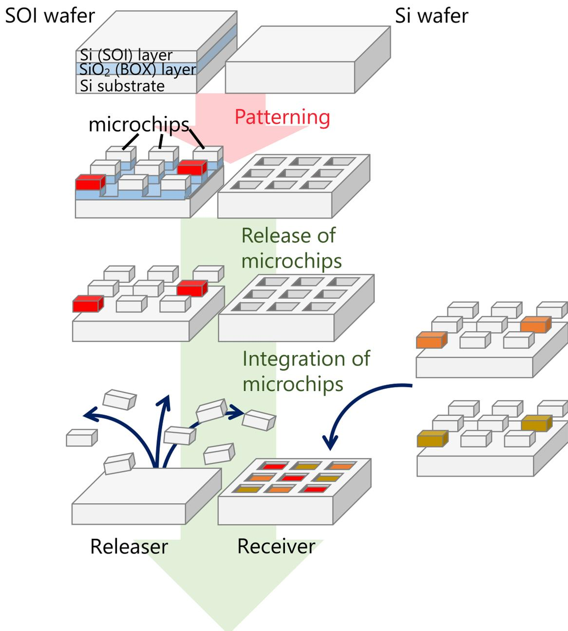
**Figure 1.** Schematic illustration of a prospective process flow of Si fluidic self-assembly. In practical applications, various-functional microchips from multiple kinds of wafers can be integrated into a single host chip. Different colors of the chips indicate different types of functions of the chips to be assembled.
