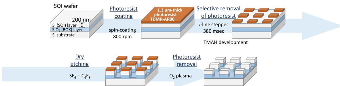
**Figure 2.** Schematic flow diagram of the fabrication process of the releaser.
