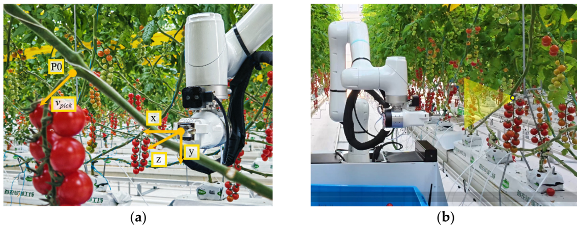
Figure 4. Coordinate system and constraints. (a) Tool frame and orientation constraint; (b) cone constraint for approach path.
