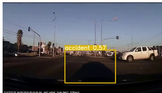
Figure 6. Example of the detection of the vehicle's shadow as the collided object.
