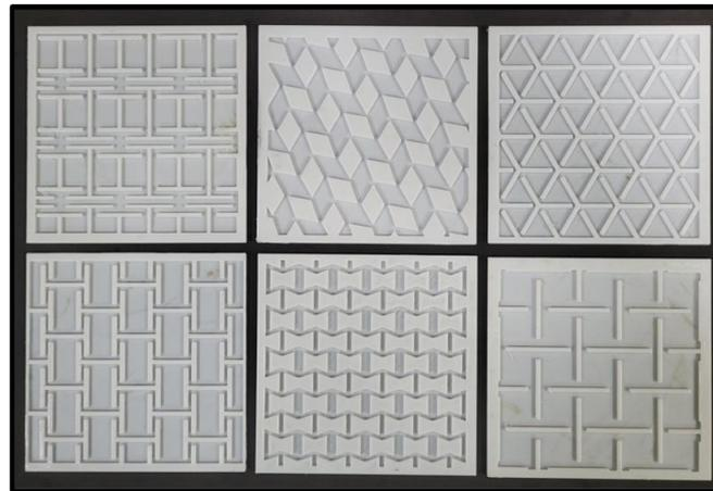
**Figure 1.** Three-dimensionally printed casting molds of skin graft models.
