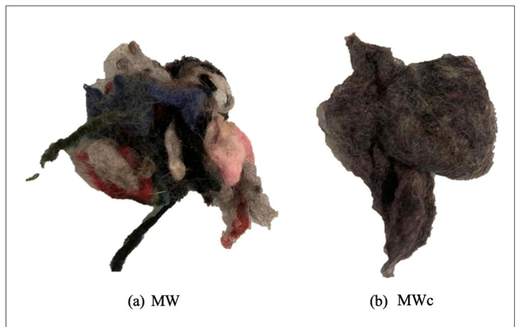
**Figure 1.** Examples of both raw material types tested. MWool<sup>®</sup> (MW, (a)) and MWool<sup>®</sup> carded (MWc, (b)).
