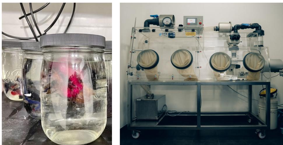
**Figure 2.** Experimental activities: representative images. Mesocosms to test MWool<sup>®</sup> degradation in marine environments (**left** Image) and box-gloves (**right** image) used to manage samples under controlled conditions used for microfibers particles analyses.
