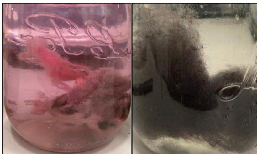
**Figure 5.** Pigment release in exposure water. In this figure, MWool® (MW, left side) is compared with MWool® carded (MWc, right side) after the same exposure time (T1). The release of pigment in contact water was recorded (MW).
