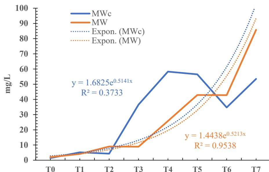
**Figure 6.** Mathematical model of release of microparticles from tested materials during the exposure time. TSS data are expressed as mg/L of microfibres released. Correlations among the model and recorded data are reported with equations as  $R^2$  values. Orange line represents MW wool, while blue line represents MWc wool. Equations are reported respectively in blue (MWc) and orange (MW) colours.
