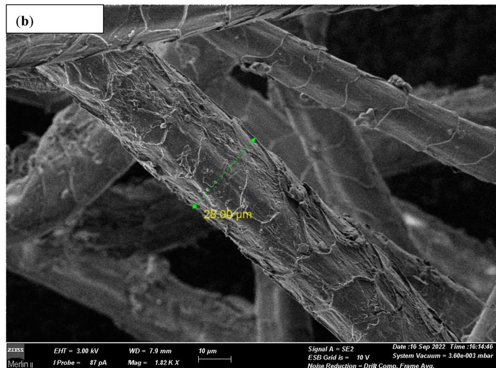
**Figure 4.** FESEM microphotographs selected for this purpose. (a) (T1) and (b) (T7) of tested MWOol<sup>®</sup> fibers with evidence of measured thickness.
