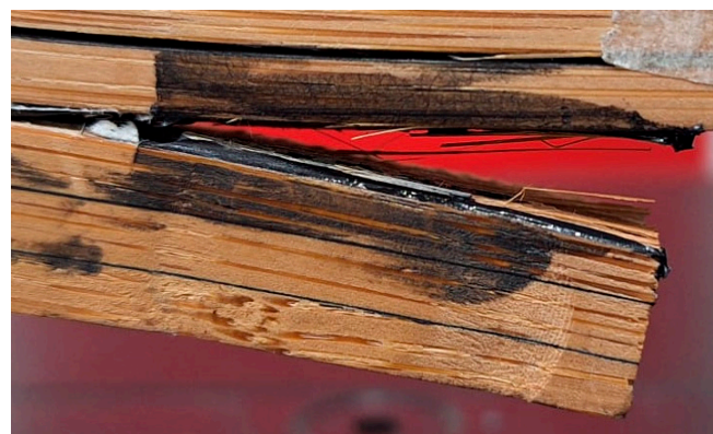
Figure 8. Detail of delamination failure of bamboo in an adhesive-only joint.
