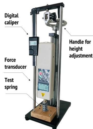
**Figure 1.** Experimental setup for the force-displacement measurement.
