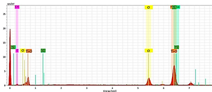
**Figure 15.** EDS-SEM analysis composition of the non-used tappers.
