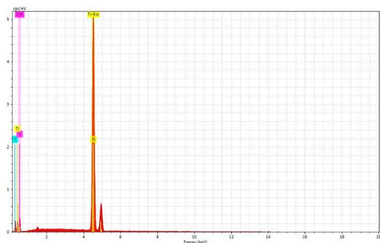
**Figure 11.** EDS-SEM analysis composition of the non-used tappers.
