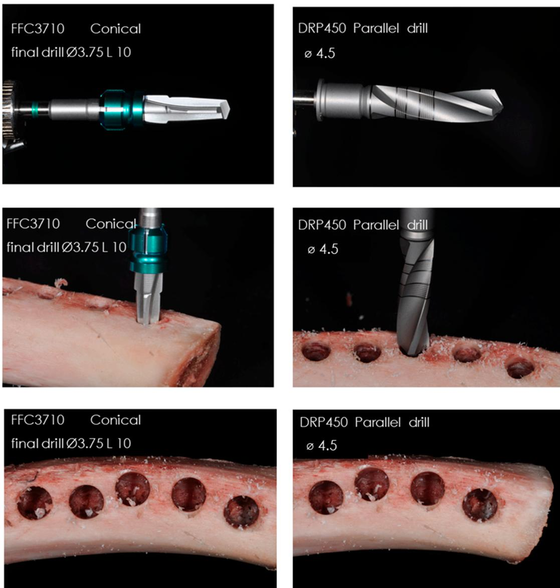
**Figure 2.** Details of the drilling sequence (continued).
