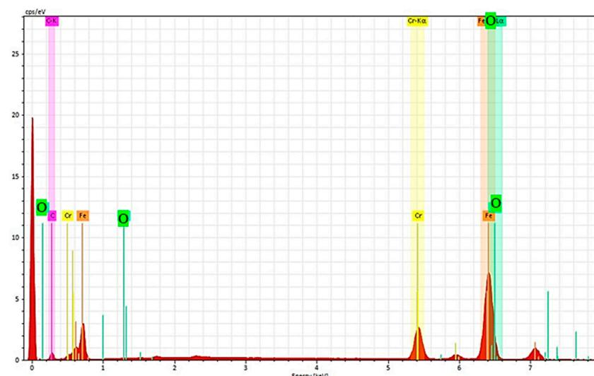
**Figure 14.** EDS-SEM analysis composition of the non-used drills.
