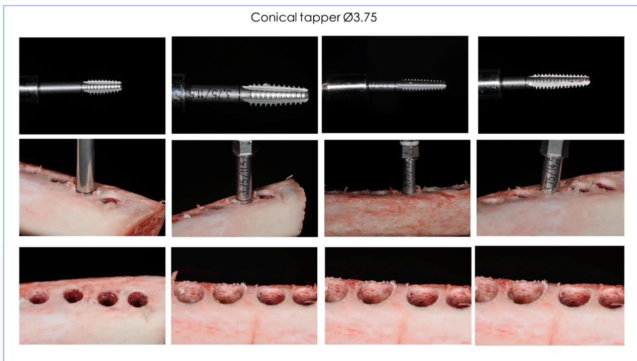
**Figure 5.** Details of the conical tappers preparation.
