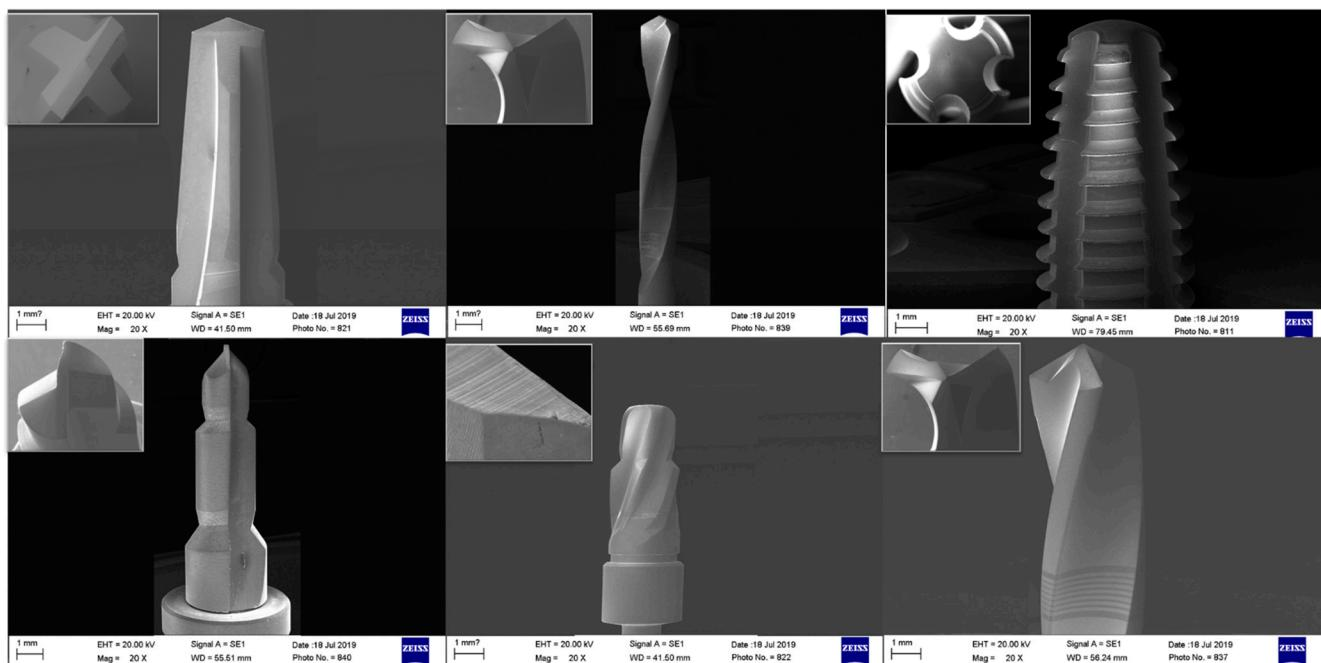
**Figure 8.** Details of the SEM analysis of the drills used in the present experiment.
