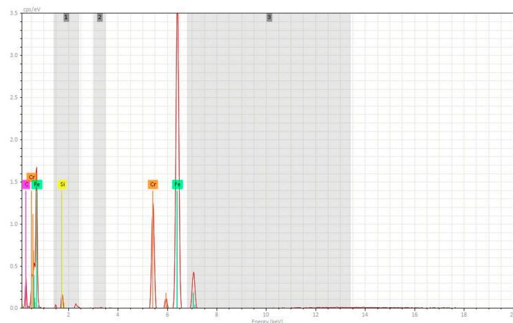
**Figure 10.** EDS-SEM analysis composition of the non-used drills.
