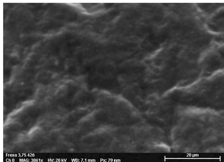
**Figure 13.** SEM analysis composition of the used drills (Mag. 3861x).
