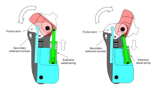
**Figure 2.** The main functional components of the variable cadence controller (VCC). **Left**: Increased friction and low spring force (and secondary extension bumper) decreases terminal impact near full extension; **Right**: Progressively increased friction (light pink area) and spring force with increase knee flexion helps to limit heel-rise and duration of swing-phase. The technical research details related to the development of the swing-phase controller can be found in [13,19].
