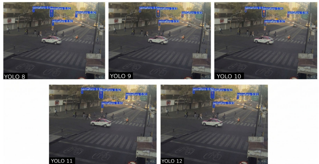
Figure 16. Real-time images used to qualitatively evaluate each trained network (traffic light detection, YOLO v8–v12).
