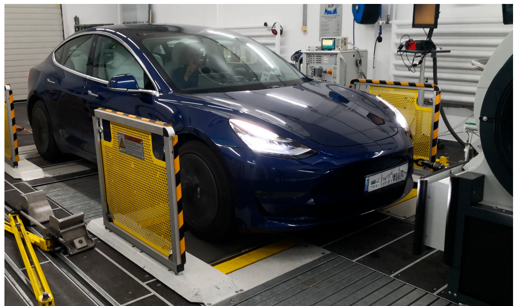
Figure 4. Test setup and road load simulation test of the EV on the chassis dynamometer.
