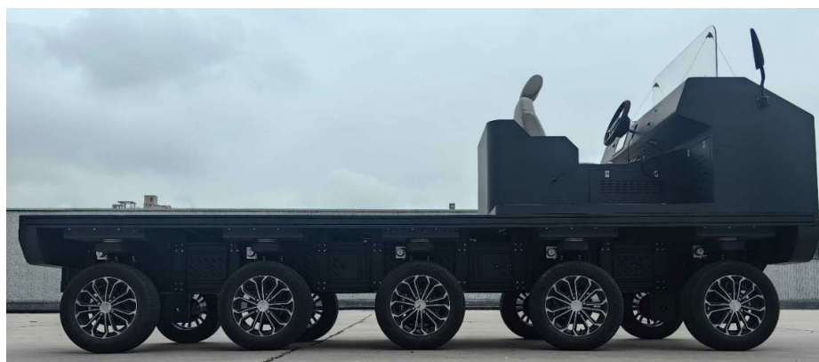
Figure 1. Distributed drive carrier experimental platform.
