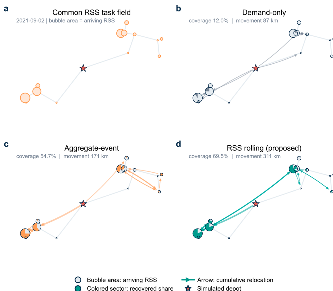
Figure 7. Spatial dispatch comparison on the same high-residual day and frozen topology. (a) The common RSS task field. (b) Demand-only dispatch. (c) Aggregate-event dispatch. (d) RSS-driven rolling dispatch. Bubble area encodes arriving RSS, the colored sector encodes recovered share, and arrows show the largest cumulative relocation flows; the pale remainder denotes unrecovered RSS. All panels share the same event stream, fleet, depot, and travel model. Coordinates are simulated and do not represent observed roads or exact station locations.
