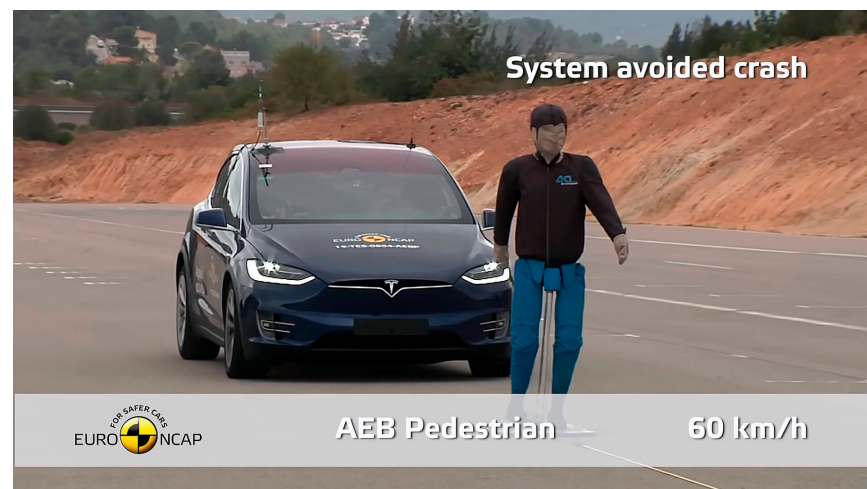
Figure 4. AEB test with pedestrian.
