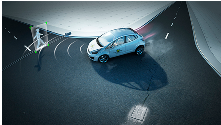
Figure 5. Visualization of the AEB test when performing a turn maneuver at an intersection.
