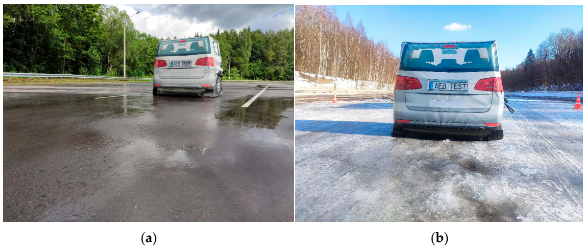
Figure 16. (a) The appearance of the target and the condition of the coating during tests on wet asphalt. (b) Appearance of the target and coating conditions during icy coating tests.
