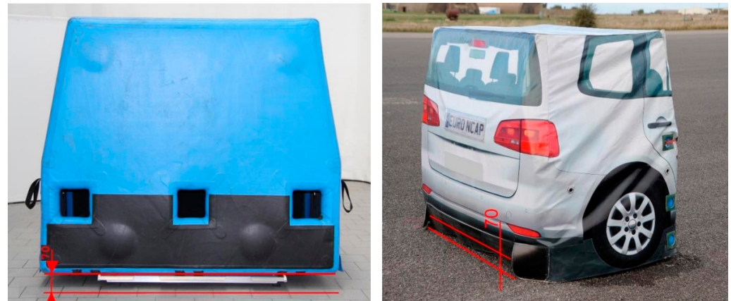
Figure 2. Target for testing at high speeds.
