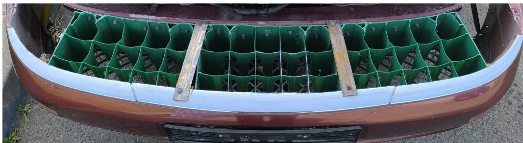
Figure 10. Plastic frame of the damping system.
