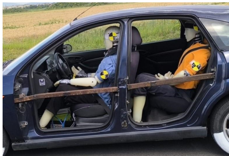
Figure 15. Positioning the dummies in the vehicle without damping.
